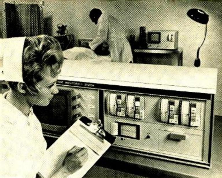
Fig. 1. Patient monitoring system gives doctor on-the-spot data and allows one nurse to monitor up to eight patients.
