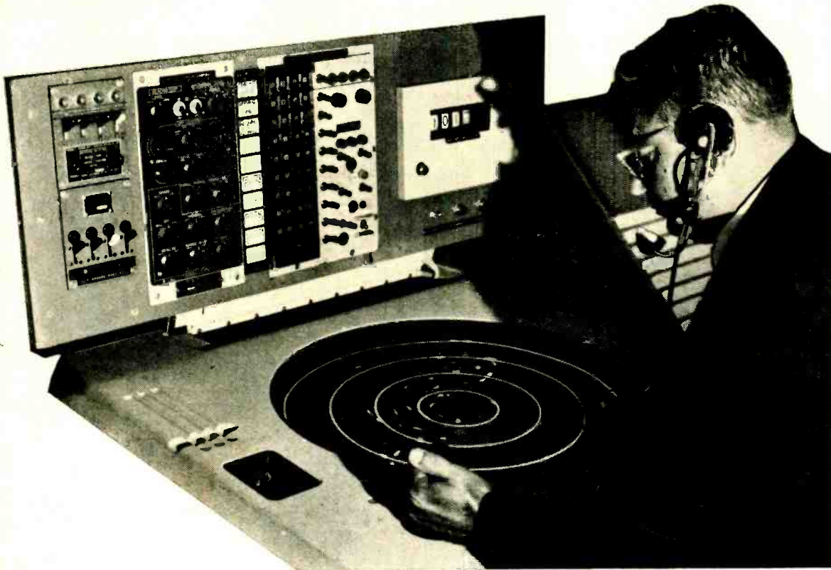
An FAA traffic controller seated at his radarscope. On the vertical panel behind the scope are the code-selector wheels along with code-assignment identifications which are employed to simplify identification of transponder-equipped aircraft.
