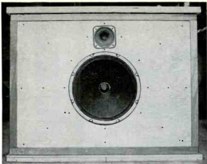
Front-panel view with speakers mounted, prior to being covered.
