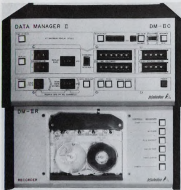
6. The front panel for a data-acquisition system typically has control switches to define the number of channels, the scan rate, the step time and many other control functions such as those for the recorder.
