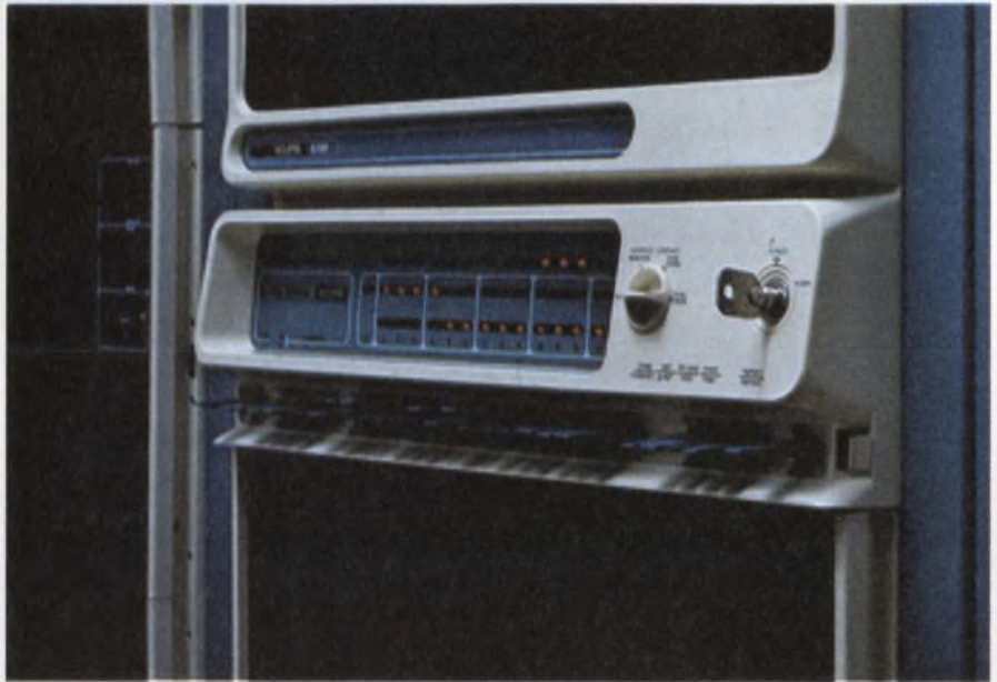
The Eclipse S/230 uses high-speed semiconductor and core-memory modules. Read cycle time for the Data General mini's 64-kbyte semiconductor memory is 500 ns, while its 32-kbyte core memory cycles in 800 ns.
