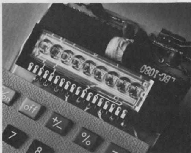
1. Built-in secondary magnification, as shown for the DL-95 LED display of a nine-digit calculator, can be used to cut drive-current requirements.
