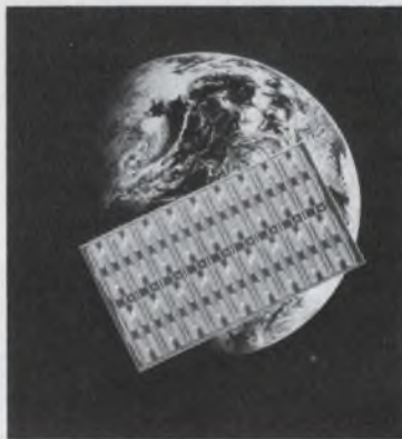
Computer-designed 248 x 140 mil chip
