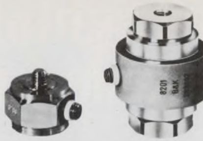
Force transducers —Models 8200 and 8201, made by B&K Instruments—can handle forces of -1000 to +5000 N or -4000 to +20,000 N, respectively.
