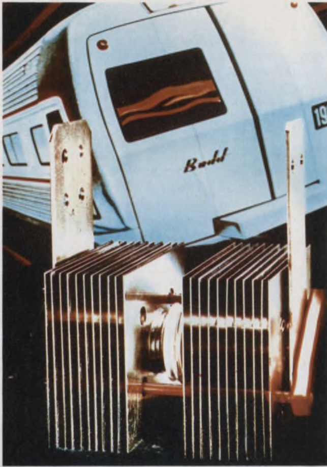
High power thyristors, like this one from Westinghouse, are finding increasing use in transportation systems.
