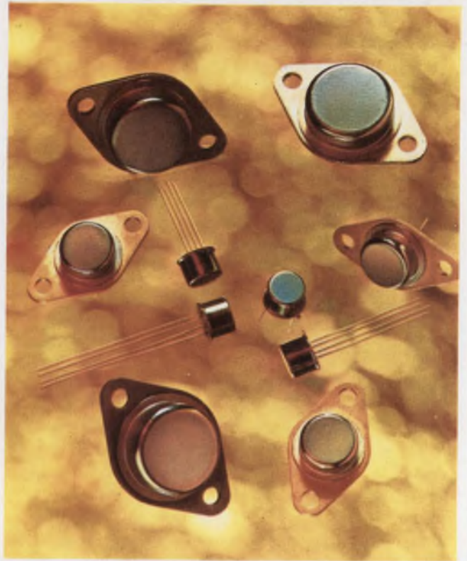
Darlington devices are gaining ground in applications formerly restricted to thyristors. Newer Darlingtons bring out the second base to form a 4-terminal device.
