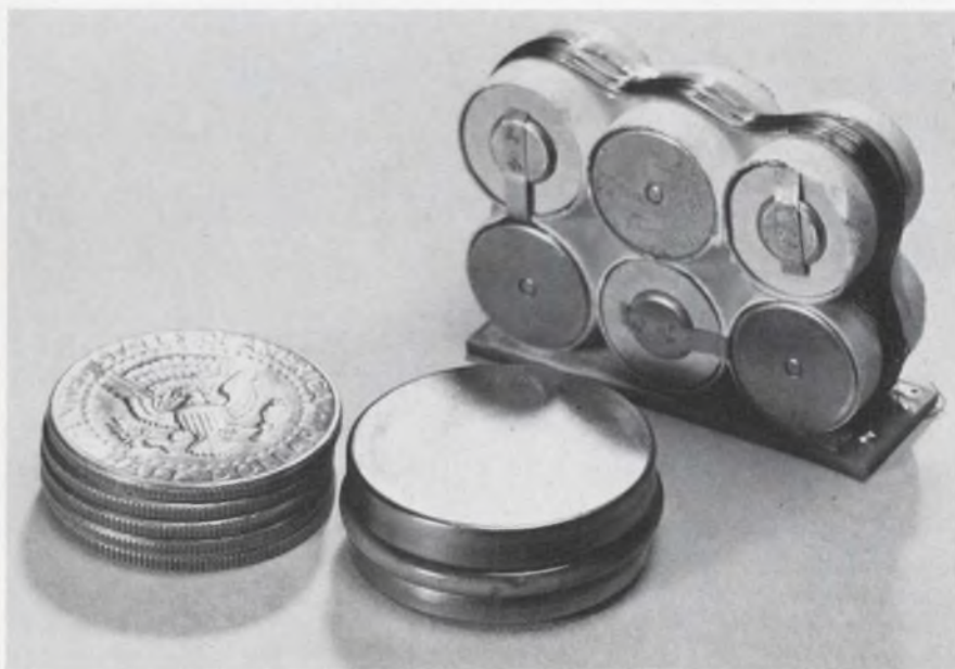
Sodium-bromine battery for heart pacemakers has a life expectancy of 10 years, equivalent to that predicted for nuclear sources.
