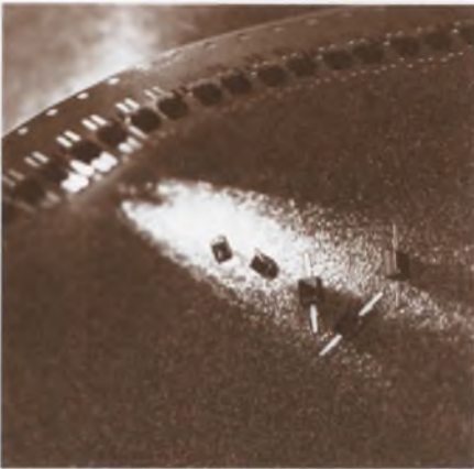
Voltage-variable and PIN diodes in a rugged new MINI-L package bring economy to tuning and bandswitching jobs.
