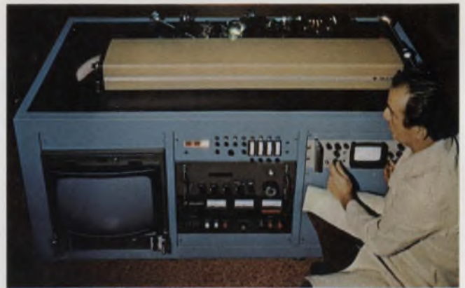
Laser color television projector, from General Telephone & Electronics Laboratories, produces pictures off the air with a single multicolor laser, single modulator and single scanner (Session 3E).
