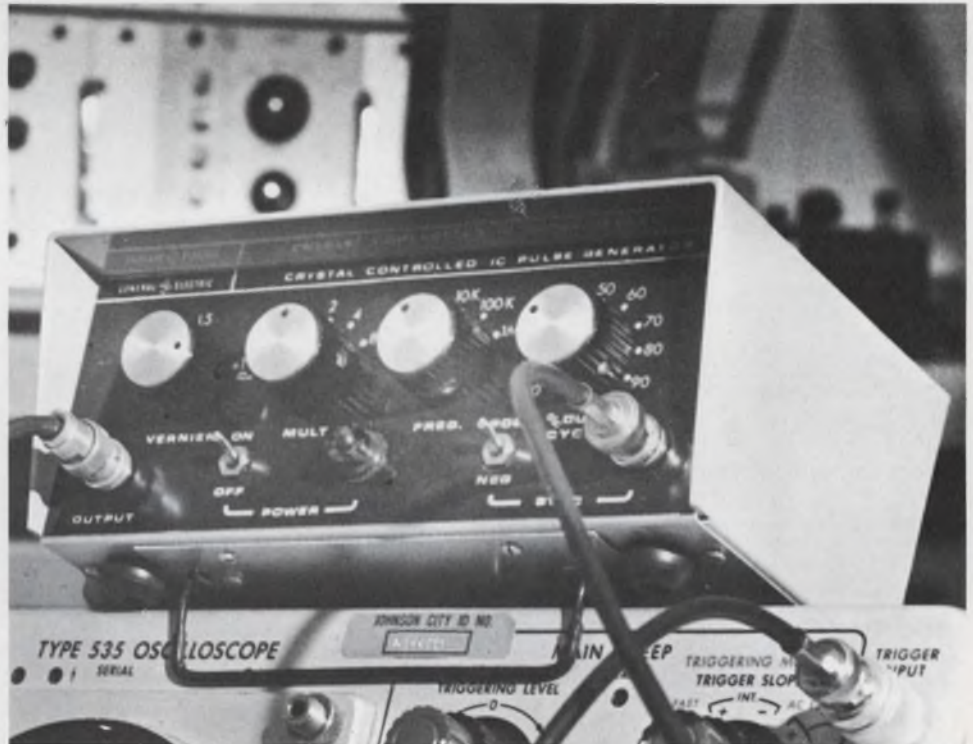
A pulse generator can be designed with ten ICs (off-the-shelf digital microcircuits) and just one crystal for stability. Page 90
