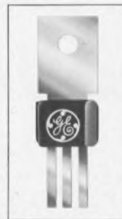
Actual size C106 SCR with flat leads and heat sink tab.
