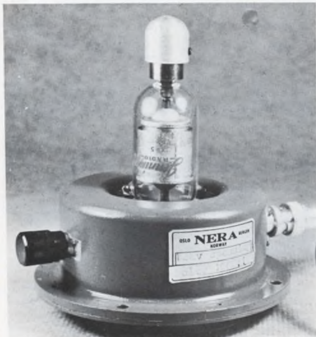
5. An accuracy of +2% is achieved with this capacitive divider by using a vacuum capacitor and a ceramic-trimmed precision mica.
