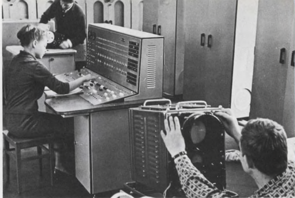
Typical small Soviet computer is the minsk-22, here undergoing checkout at a factory in Minsk. (Novosti from Sovfoto).
