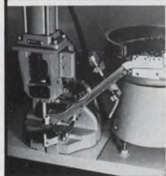
This automatic machine was developed to assemble Clinch-Loc Terminals with speed and flexibility for volume users. With an alternate track any Clinch-Loc Terminal can be used in this machine.
