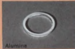
Alumina O.D. .604 ± .005 I.D. .510 ± .005 Thickness .040 ± .005 Wall Thickness .047 ± .0015
