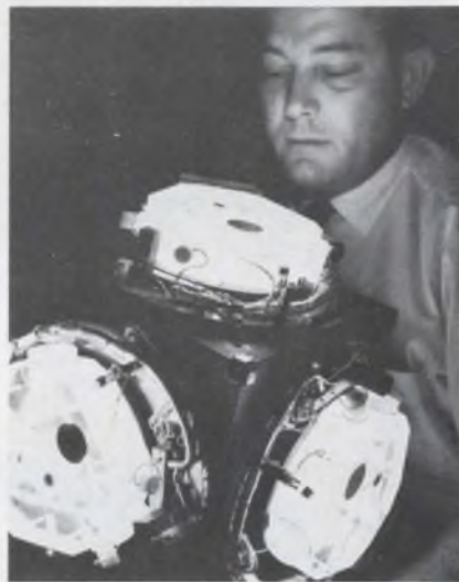
Three-axis laser gyroscope uses mechanical biasing to keep beams from locking in phase at very low rates of rotation.
