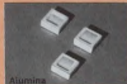
Alumina O.D. .220 ± .002 Square Thickness .030 ± .002 Counter Bore Depth .025 + .005 - .000 Counter Bore Dia. .175 ± .002
