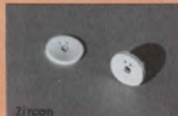
Zircon Thickness .030 ± .002 I.D. .060 ± .001 Two Holes .020 ± .002 Hole Center .054 ± .002 O.D. .273 ± .001 Ground
