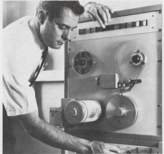
Solid-state spectrograph prints taped sound pictures in a matter of seconds. Page 20
