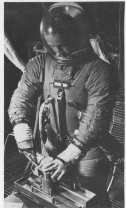
Astronaut uses electron-beam gun to weld stainless steel in chamber that simulates conditions 380,000 feet up.
