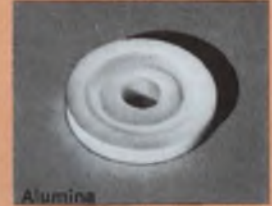
Alumina O.D. .800 ± .005 Boss O.D. .400 ± .005 Counter Bore Depth .020 + .005 - .000
