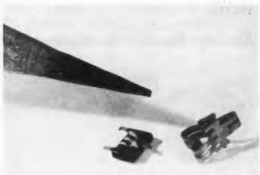
One-piece connector used in Thompson Ramo Woolridge micromin system is shown with microtransistor. Pencil point provides scale.
