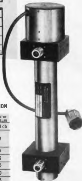
Model M2105 Low Noise TWT weighs 5 pounds and is 12 1/8" long.
