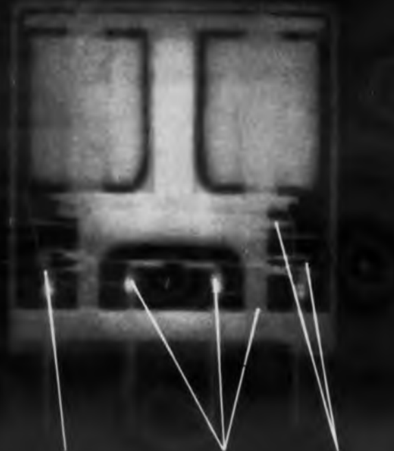
Contacts positively carried—no spring bias All-welded coil leads, contacts and frame supports Matched-action armature and contact structure
