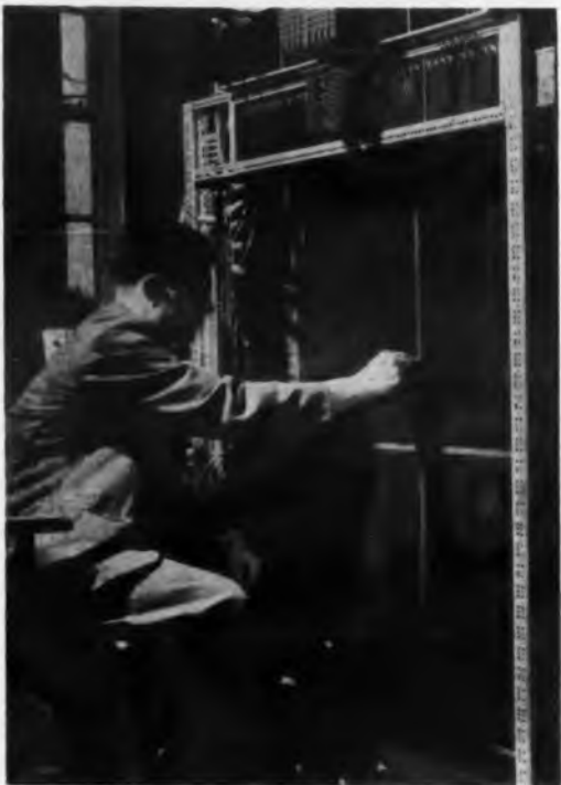
Ferrite-rod, wire-mesh memory of experimental version of Atlas computer contains fixed instructions and computes on basis of information supplied by slower memories in system. Its access time is said to be 0.3 \mu sec. An Atlas designer, Dr. R. L. Grimsdale, Manchester University, adjusts a ferrite rod in wire matrix.
