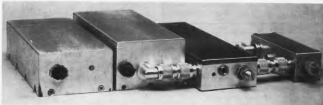
Complete parametric multiplier package developed by Pacific Semiconductors, Inc. and Space Technology Laboratories delivers 2.5 w at 2.25 Gc. From left to right: crystal-controlled 94-mc oscillator and preamp; transistorized amplifier with 13-w output; tripler and two successive doubler stages delivering 4 w at 1.1 Gc; final doubler stage.
