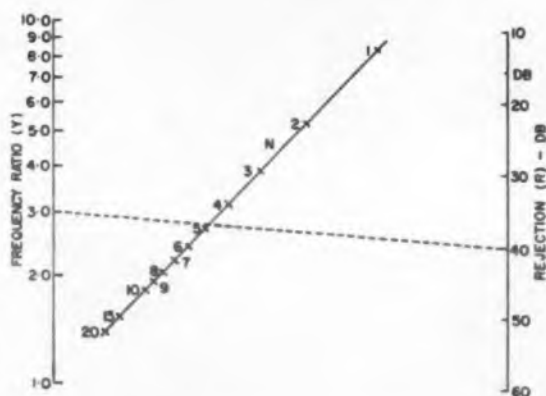
Fig. 2. Cavity nomogram for symmetrical band-pass filters.
