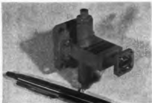
Typical harmonic generator built by Microwave Associates. This model 799C employs 500-mw 11-Gc input to deliver 33 Gc output with 20 db conversion loss. Device incorporates input and output filters.
