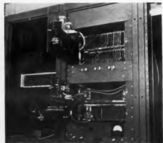
Data-processing section of system has punch-control circuitry, top; digital clock showing Nixie tubes; an analog-to-digital converter, shown open; and a logarithmic amplifier to compress the 30-db dynamic range of incoming signals so they can be handled by an analog-to-digital converter.
