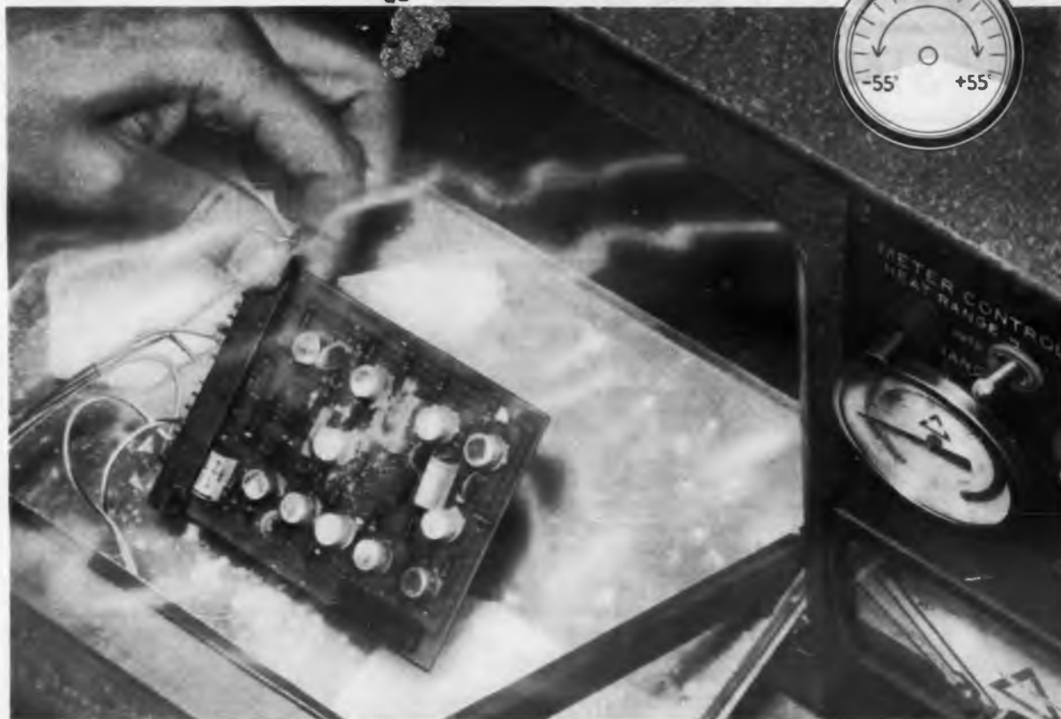
NEW DONNER OPERATIONAL AMPLIFIER features exceptionally low drift with temperature variation. (See specs below.) Single channel Model 3811 shown here was tested between -55^{\circ}\text{C} and +55^{\circ}\text{C} in temperature chamber—standard procedure for all Donner amplifiers before delivery.
