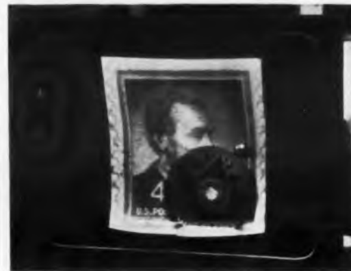
Close-up of television-comparator monitor shows full-screen view of postage stamp, printed-circuit disk, and pin head. Magnification is about 10 to 1.
