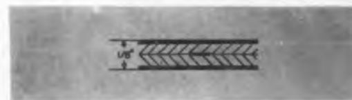
Fig. 4. Triplate line is self-supporting and is available in considerably smaller sizes than other strip lines. Attenuation is increased, however, because of dissipation in the dielectric.
