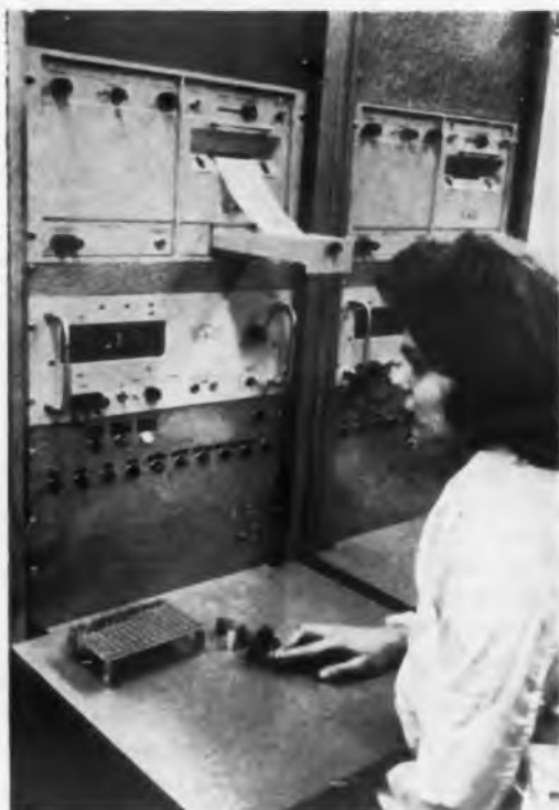
Fig. 4. Human errors in reading and recording the enormous amount of data involved in reliability testing could greatly affect the final failure figures. Thus, an additional refinement, to enhance the reliability program, involves the design and installation of automatic recording equipment. An automatic set-up for reading and recording transistor test data is shown. (Photo courtesy of General Instrument Corp.)
