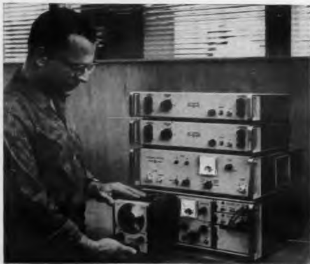
Grooved feet allow for easy, stable stacking. Sub-modules can be grouped together in modular adapters so they can be stacked with full-width instruments or mounted in racks.
