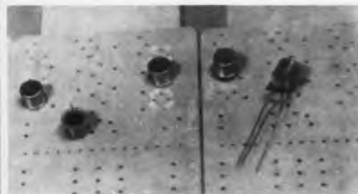
Embossed ridges on PC card at left serve as transistor mounts instead of washers shown at right.
