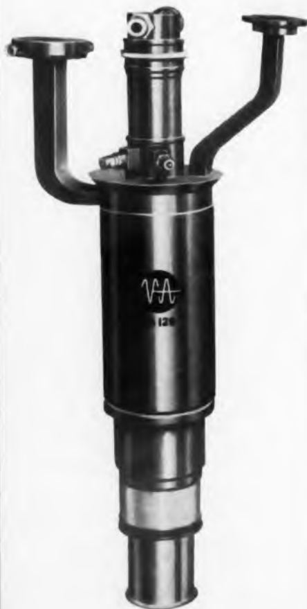
VA-126 TWT 3 MW Peak 5 KW Average 5.4 to 5.9 kMc
