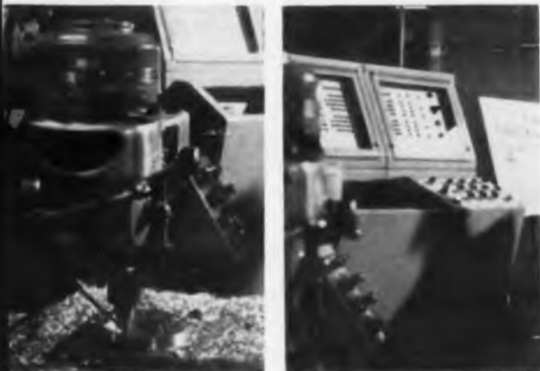
Thompson Ramo Wooldridge's three-axis contour control shown directing a Gorton rail mill.
