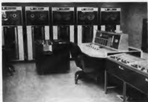
Main console , right, and several tape units of the $3 million IBM 7090 computer used as the hub of Socony Mobil's growing business-automation system. The company hopes to improve the integration of its facilities throughout the world with real-time data communications networks over the next few years.
