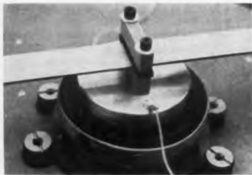
. . . can be mounted quickly without need for bolting specimen down.
