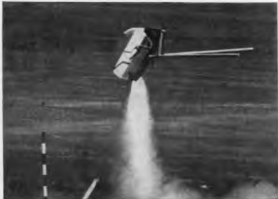
The photo above shows an ejection seat being catapulted from the sled on which the camera control unit is mounted. The test dramatically illustrates the extreme forces and vibrations to which the unit is subjected. Another example of advanced equipment design made possible by the use of General Electric SCR's.
