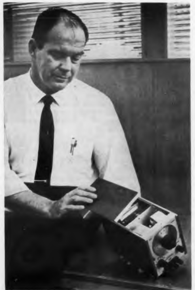
Top and bottom covers, as well as side plates, snap off for easy access to components.
