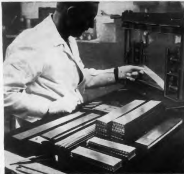
UAP worker assembles multiple parts in fixture for heat exchanger core. Gloves guard against contamination of aluminum prior to brazing.
