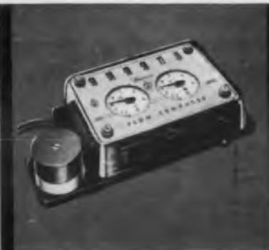
Flow Computer ... extracts square root and continuously integrates both differential and static pressures for applications such as orifice measurement of fluids.
