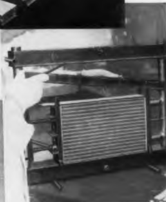
Fixturing is complete. Assembly proceeds rapidly since bonding of parts is achieved in a single dip-brazing operation.
