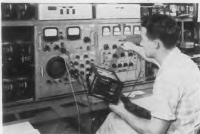
Precise evaluation of highly complex electronics armament systems requires that manufacturing engineers design and develop test equipment frequently as complex as the system being tested.
