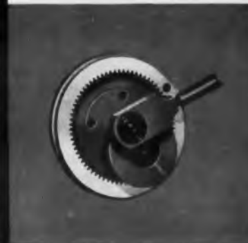
Sine Cosine Mechanism ... for problems of changing variables involving vector components, range and bearing computations, sight computation, etc.
