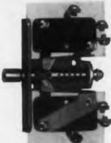
MODEL C2-7 Solid shaft. D.P.D.T. Pre-travel: 3/16" max. Elec. rating: 10 amp. 125/250 V.A.C. 60 cycle. Amb. temp.: -100° to + 275° F. Elec. & Mech. Life: 150,000 ops. Dimensions: 2-3/32" x 1 7/8" x 33/64"
