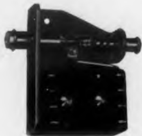
MODEL C2-9 D.P.D.T. Elec. rating: 15 amp. 125/250 V.A.C. 60 cycle. Oper. force: 4 3/4 lbs. ± 12 oz. Amb. temp.: -100° to + 275° F. Elec. & Mech. Life: 150,000 ops. Weight: 2 oz. approx. Dimensions: 1-29/32" x 1-31/32" x 9/16"
