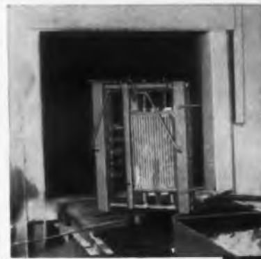
Pre-heat furnace assures 100% heat penetration of fixtured assembly prior to immersion in flux bath.
