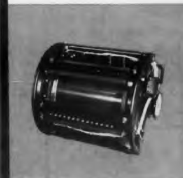
Magnetic Storage Drum ... for medium storage applications; capacity 131, 072 non-volatile bits; drum speed 3800 rpm; clock frequency 130 kc.
