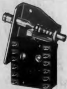
MODEL C2-14 T.P.D.T., 6 ckt. Pre-travel: 5/32" min. Overtravel: 1/4" approx. Mov. Diff. .028" ± .007" Elec. rating: 15 amp. 125/250 V.A.C.—15 amp. 30 V.D.C., res.—10 amp. 30 V.D.C., ind. Life—500,000 ops. min. Dimensions: 2-5/16" x 1-31/32" x 9/16"
