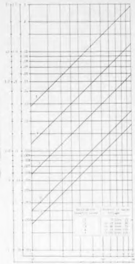
Curve 13. Paper capacitors, equipment failures as a function of application severity. Vitro .
