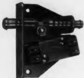
MODEL C2-4 S.P.D.T., 2 ckt. Elec. rating: 125/250 V.A.C., 30 V.D.C. —10 amps. 125 V.D.C., 1/2 amp. 250 V.D.C., 1/4 amp. Oper. force: 2 lbs. ± 12 oz. Weight: 2 oz. Dimensions: 1-13/16" x 1-31/32" x 9/16"
