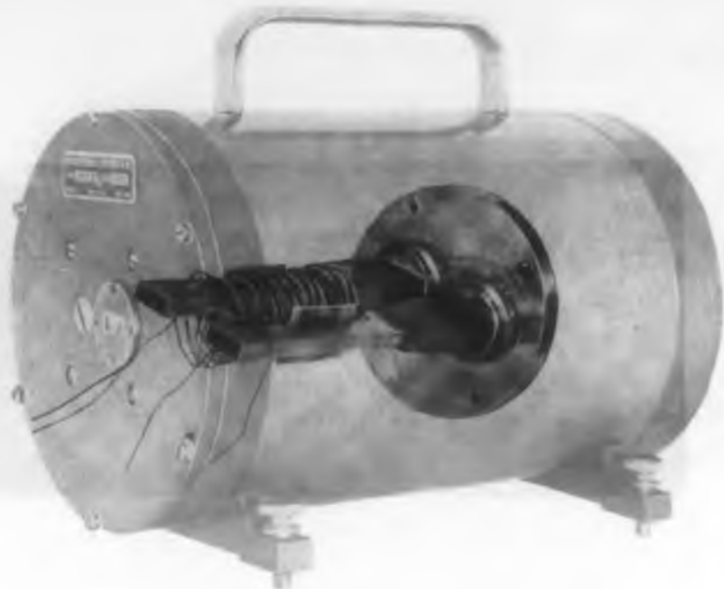
Internal view of dry calorimeter showing active and reference waveguide and thermopile.
