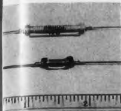
△ High Ambient Resistors Carbon on Ceramic
