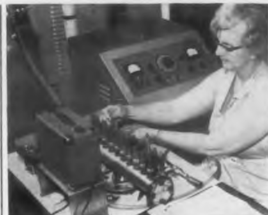
TESTING TRANSISTORS in electronic equipment is one of many uses for the versatile M2 leak detector, shown in background.
