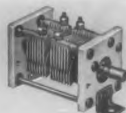
"VU" Permits use of "lumped constant" circuits up to 500 MC. Two sections in series eliminate rotor wiper. Pyrex glass ball bearings eliminate noise from usual metal-to-metal bearings.
