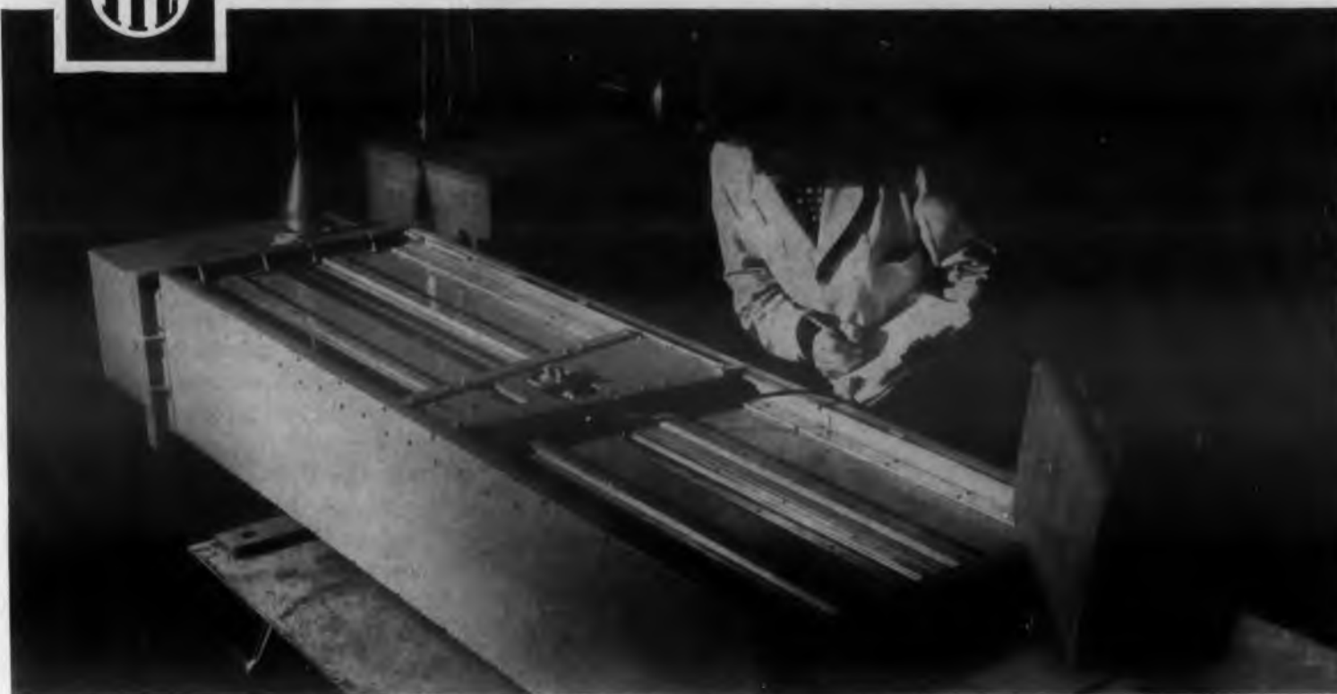
Slotted line for waveguide size WR 2100. Covers range of 350-530 mc. Probes tunable over entire band. Inherent VSWR less than 1.02--slope less than 1.01. Features bolted and doweled aluminum construction.
