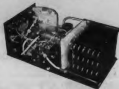
MODEL MB-177, TYPE 202 DISSIPATION: 1700 watts. ALTITUDE RANGE: sea level to 50,000 feet. POWER REQUIRED: 110 volt, 400 cycle, 3 phase. WEIGHT: 27 pounds. SIZE: 10" x 19 15/32" x 7 1/2" high, per JAN-C-1720A, size B1-D1.
