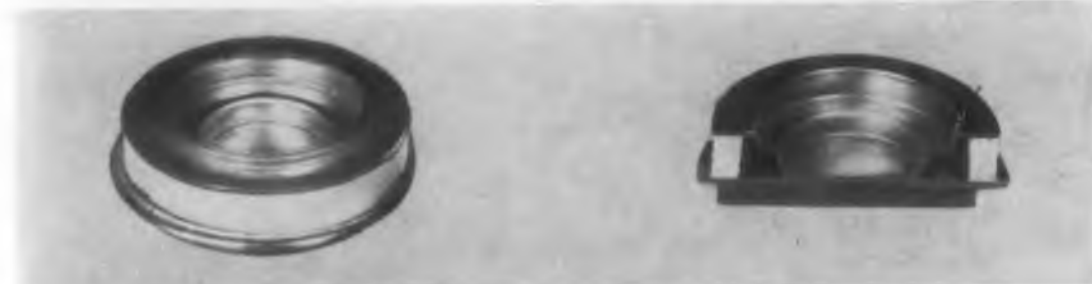
ACTUAL SIZE OF G-E germanium and silicon rectifier cell, hermetically sealed in ceramic housing, is shown in side view (left) and cutaway (right).
