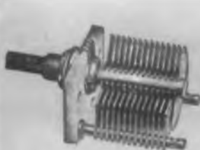
"MFA" Similar to "HF" model, but with larger air gaps for higher breakdown ratings. Used for high-frequency, low-power transmitting. Also available as dual unit.
