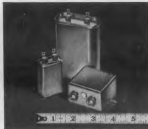
PERMAFIL RECTANGULAR solid dielectric in case styles CP50, CP60, and CP70 series. Built to electrical requirements of characteristic "K", MIL-C-25A. Ratings: .01 uf to 10 uf; 100 v. d-c to 1500 v. d-c, Temp. range: -55C to +125C.
