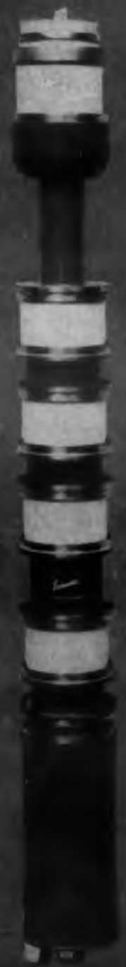
4K50,000LQ Four cavity klystron that delivers 10,000 watts of power at frequencies of 700 to 1000 MC
