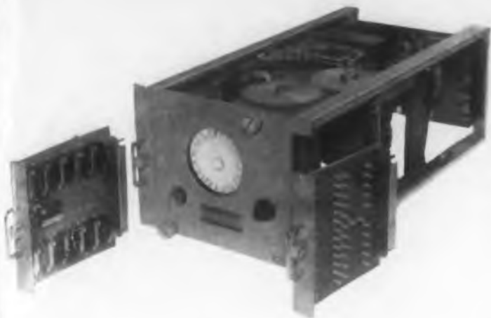
Typical servo showing plug-in padding turrets with adjustable load resistors.
