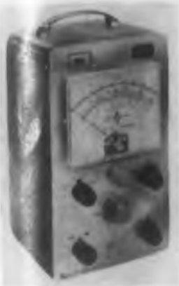
△ Transistor Tester Self-Contained Unit
