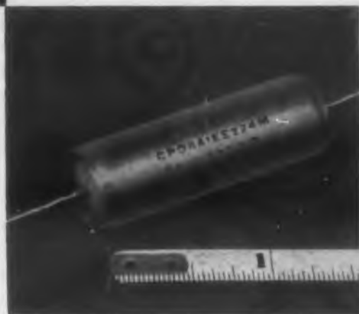
METAL-CLAD TUBULAR CAPACITORS — +85C, mineral oil impregnated. Built to MIL-C-25A. Ratings: .001 to 1.0 uf, 100-600 v. d-c. Tol: \pm 5\% , \pm 10\% , or \pm 20\% . Write for GEC-1390.
