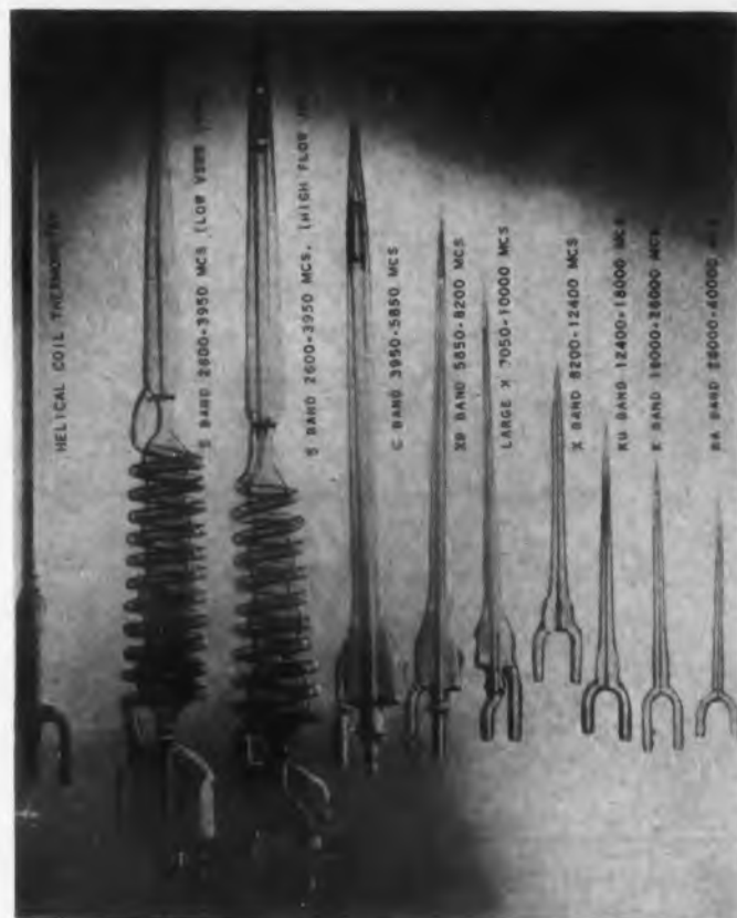
Fig. 2. Calorimeter waveguide loads for dominant mode operation between 2600 and 40,000 megacycles. Thermometer is shown at left.
