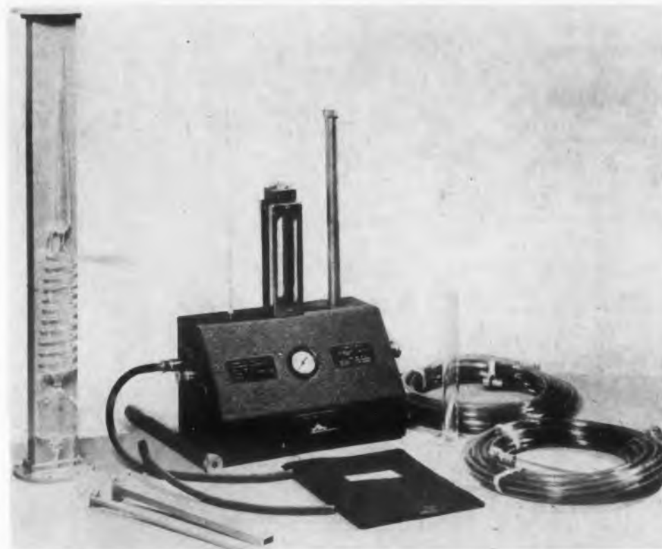
Fig. 1. Complete RF Calorimeter System for water tap operation. Power capability is unlimited. May be used with either waveguide or coaxial lines from vhf to higher frequencies.
