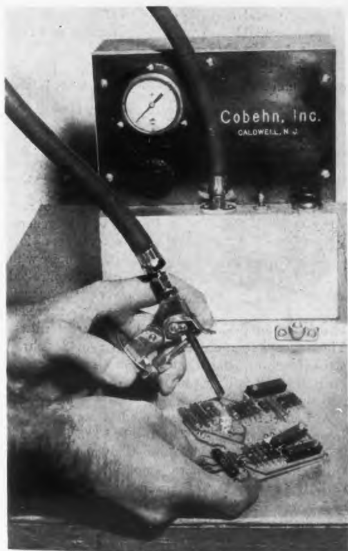
Cleaning electronic assembly with high-velocity solvent spray
