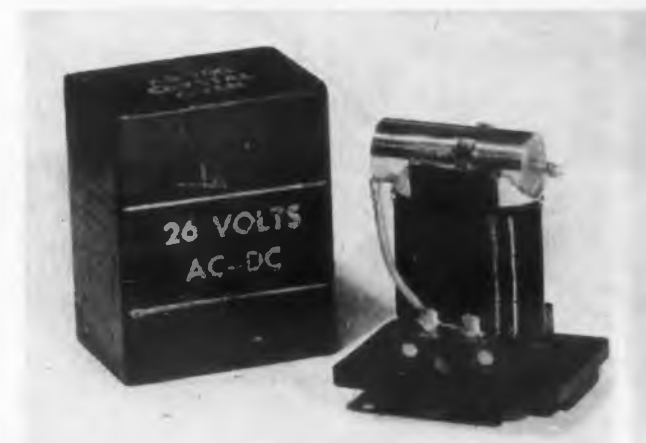
Shown is a partially-assembled crystal oven with thermostat mounted and wired for operation as used by Bulova.
