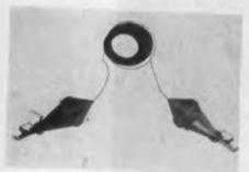
The G-Line is a new economical single wire surface wave transmission line assembly designed to eliminate coaxial transmission line
