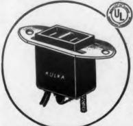
No. 221 (above) with soldering terminals and steel bracket with #6 clearance mounting holes. Also No. 222 with 6-32 tapped mounting holes. No. 223 (left) with 8" #14 or #16 plastic wire leads and steel bracket with #6 clearance mounting holes. Also No. 224 with 6-32 tapped mounting holes.
