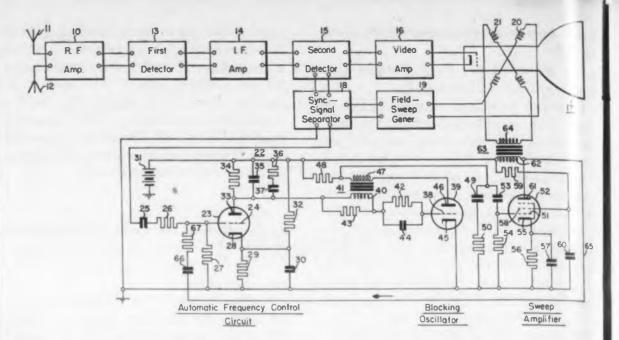
**Automatic Frequency-Control Circuit**
