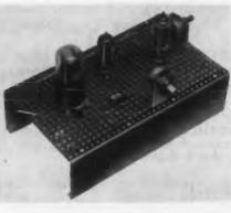
The "Experimenter's Chassis" kit provides quick set-up of electronic circuitry with simple hand tools. Although intended mainly for mockups, it is also suitable for more
