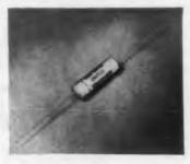
This ceramic-encased paper tubular capacitor incorporates a newly developed thermosetting plastic end seal. It will pass humidity tests at 90-95 per cent humidity over a period of 750 hr at 40 C, 500 hr at 50 C,
