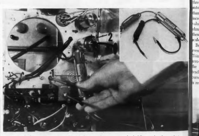
Fig. 1. Operator tests signal level in horizontal-output stage by holding probe tip against glass wall of tube. The probe (inset) converts any 20,000 ohms-per volt meter into a signal tracer.
