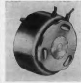
The smallest of eight basic sizes, the Model BD1E rotary solenoid weighs 1-1/2 oz and has a diameter of 1 in. Starting torques for the entire line now range from 0.2 lb-in. for the new size to 54 lb-in., based on ampere-turns for
