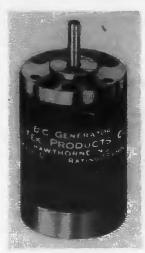
A line of low cost dc tachometer generators is offered with diameter of 1 1/8 in. and weight slightly more than 3 oz. Although used principally as rate generators in servo systems, these units have many other uses. When combined with a standard 1000 ohms/v voltmeter, they make an excellent direct-reading tachometer. They can be used as under or over speed indicators, speed synchronizing
