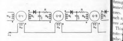
Fig. 5. One core per bit transfer loop.
