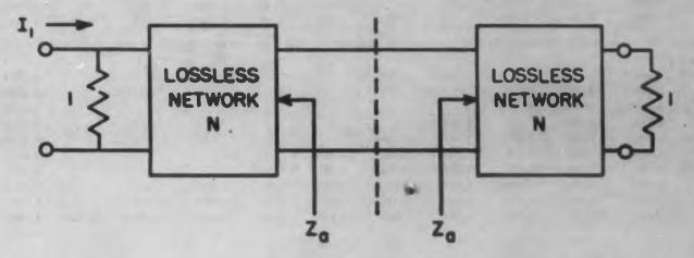
Fig. 1-3 Decomposition of a symmetrical network into two network halves.
