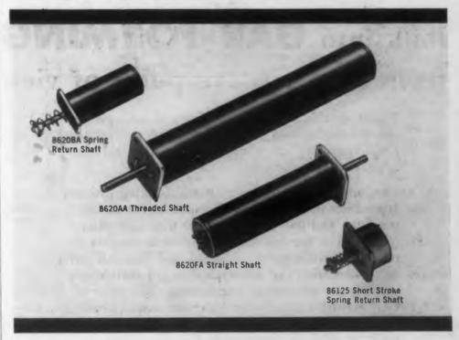
Resistance Ranges — from 80 ohms to 75000 ohms per inch of stroke Linearity — better than  $\pm 0.5\%$  of total resistance Resolution — as high as 0.001 inch Shaft Displacement - from 0.1 inch to 5.0 inches
