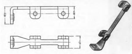
PROBLEM – Brackets which meet military specifications for vibration and shock are required for mounting terminal boards or printed circuit panels.
