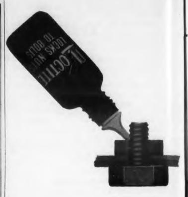
THREADED fasteners can be vibrationproofed with a new liquid sealant. Heavy vibration does not loosen the locking action but simple torque tools easily separate the threaded hardware.
