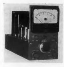
The Type 67 Universal Control System is a complete, miniaturized carrier measurement tem available in various models to operate all types of transducers, including variable permeance, variable reluctance, variable dif-
