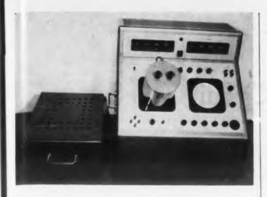
a damping counter consisting of the necessary trigger tubes and electrostatic, highvacuum decade counter tubes.
