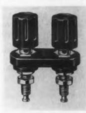
This mounting base is used for quick assembly of two binding posts to make a dual unit. It is designed to receive the Model No. 29-1 Binding Post having a OD of only 1/2 in., and for 3/8 in. mounting holes on 3/4 in. centers. It is available in red or black thermosetting phenolic
