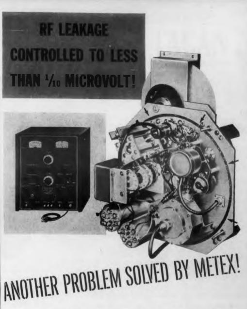
This Type 240-A Sweep Signal Generator built by Boonton Radio Corp., Boonton, N. J., is designed to operate at controlled output levels down to 1/10 microvolt. To prevent RF leakage between the oscillator chassis and oscillator cover, Boonton engineers specified a METEX RF gasket at this critical joint. This METEX RF gasket, knitted of monel wire, prevents RF leakage so successfully that peak performance is obtained at minimum output levels where leakage was previously experienced.
