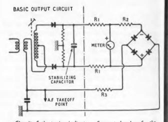
Circuit of the tuning indicator. Suggested values for the resistors (all 1-W) are:-
