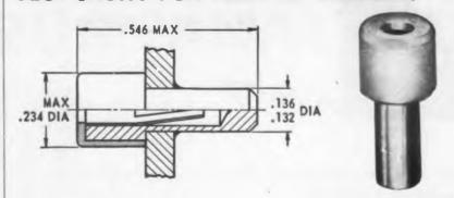
PROBLEM - Convenient test points are needed on printed circuit panels. Jacks must lend themselves to easy assembly and automatic dip soldering.
