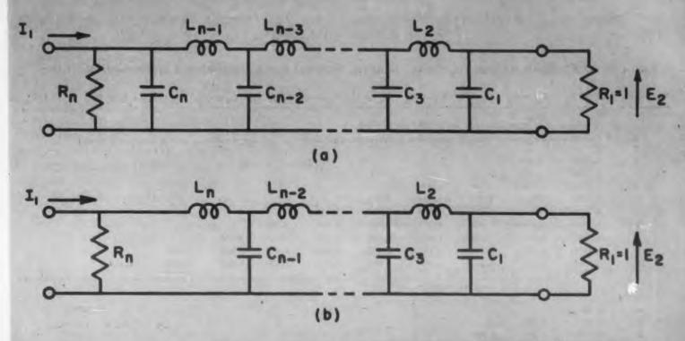
Fig. 1-1 General forms of low-pass ladder network with a current-source input and resistance terminations at both ends.
