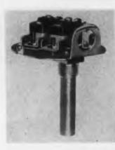
Two independent electrical circuits can be controlled simultaneously with the Series 22000 dual-control "Thermoswitch." Basically, this thermostat consists of a liquid-filled sensing element, containing a sensitive bellowsand-push-rod assembly which actuates two precision miniature snap
