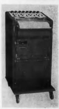
Space-saving compactness and mobility are two features of a new 8-channel oscillographic recording system. Completely selfcontained, the Model 158-5490 system is designed primarily for recording analog computer outputs, but may also be used for other types of recording. Over-all, the new system measures only 46-1/2 in. high, 27 in. deep and 22 in.
