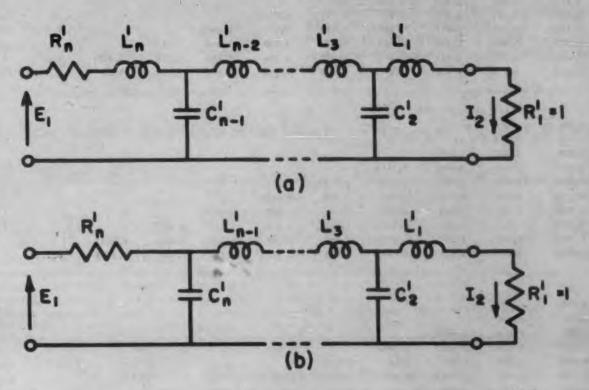
Fig. 1-2 General forms of low-pass ladder network with a voltage-source input and resistance terminations at both ends.
