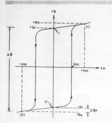
Fig. 1. Hysteresis loop of ferromagnetic core material.
