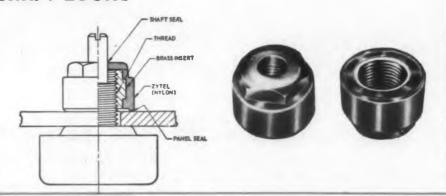
PROBLEM -To retain adjustment of slotted shaft potentiometers under conditions of vibration and shock.
