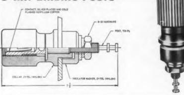
PROBLEM—A compact, high-strength binding post incorporating a test jack is required.
