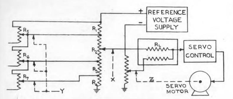
Fig. 1. Simplified circuit diagram of an electrical three-dimensional cam
