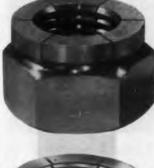
Regular FLEXLOCS are onepiece, all-metal, standard height nuts that lock securely, even under extreme vibration. Thin nuts have the same one-piece, all-metal construction and the same positive locking principle, but these nuts are approximately 30% thinner. Your FLEXLOC industrial distributor stocks both types: regular FLEXLOCS in sizes from #0 to 2"; thin FLEXLOCS in sizes from #6 to 11/2". Ask him for catalog information and samples. Or write STANDARD PRESSED STEEL Co., Jenkintown 12, Pa.
