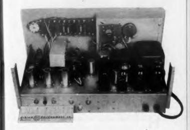
The circuit also incorporates a phase inverting amplifier, phase network driving amplifiers, a phase shifting network, cathode followers and output amplifiers. Printed circuits and miniature components are employed which result in a small packaged unit.
