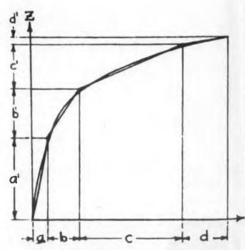
Fig. 2. Shaft rotation x versus output Z. This curve represents a cross-section of a three-dimensional cam at a point y.
