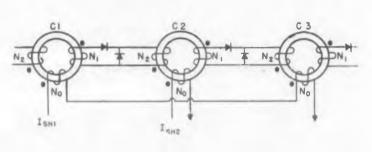
Fig. 3. Shunt diode, two core per bit shift register.
