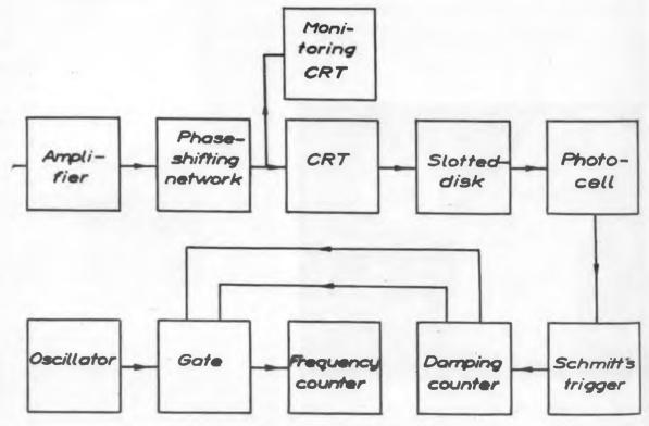
Block diagram of the Dampometer.
