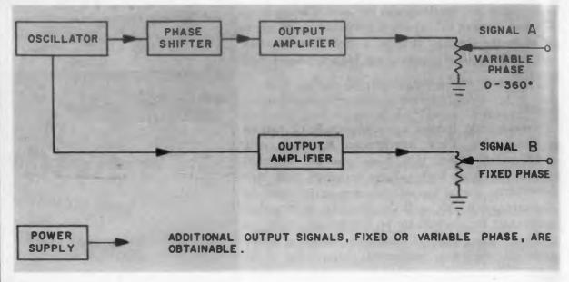
F EATURING an unusually wide frequency range, 0.2 cps to 20 kc, this Variphase Oscillator has two independent signal outputs of the same frequency but with controllable relative phase.
