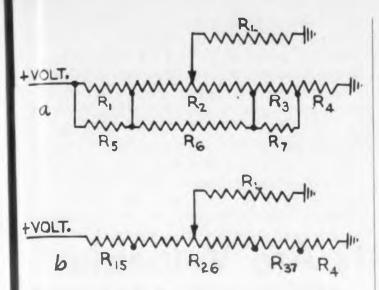
Fig. 3. Heart of the three-dimensional cam circuit is the tapped potentiometer (a). Its equivalent circuit, (b), is used to calculate resistance values between taps.
