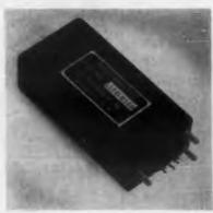
Primarily intended to receive signals from a synchro control transformer, and to operate a size 15, 400 cycle, 6.1 w servo motor or equivalent, this new servo amplifier is designed to meet the environmental
