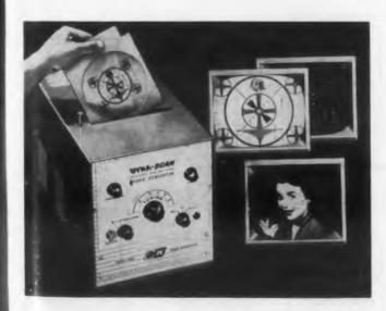
Standard or self made patterns easily inserted in Dyna-Scan for viewing on video screen
