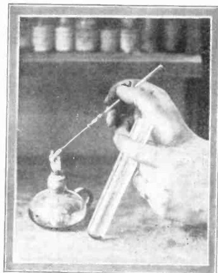
Dilute the alcoholic distillate with 5 cc of water, keep test tube cold, and plunge a spiral of red hot copper wire into the tube.
