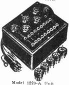
Model 1220-A Unit For servicing sets using metal, glass-metal or glass tubes. Has five sockets—with standard RMA markings. Panel also includes eight automatic switch type and ten single action jacks. Makes all series and parallel meter connections through the set sockets to all parts of the circuit. Automatic in operation. Used in conjunction with 1200 Series Volt-Ohm-Milliammeters. Extra connections may be added, when necessary, at a very slight cost. Shpg. wt. 8 lbs.
