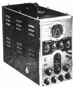
This instrument offers complete facilities for countless problems of receiver circuit study and adjustment. R.F. and I.F. alignment, resistor, condenser, and vibrator tests are made while the receiver is under actual operation.
