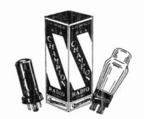
Resistance units enclosed in Radio Tube envelopes and with Radio Tube bases, are now standard for voltage reduction purposes and to supply proper voltage to pilot lamps in AC-DC receivers. With their use fire hazard is reduced to a minimum and the use of separate resistors for pilot lamps is eliminated.
