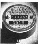
The type LD2 amateur frequency crystal is a mounted, precision low drift crystal for the 80 and 160-meter amateur bands. The crystal is carefully cut from selected Brazilian Quartz, ground to exacting precision, accurately calibrated and rigidly tested. It possesses unusual activity and has a frequency drift of less than 4 cycles/MC./°C.
