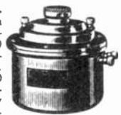
6-8 volt field excitation. 1.1 ampere consumption at 6 volts. 15-ohm voice-coil impedance at 1000 cycles. Continuous operating capacity 20 watts. Peak load capacity 50 watts. Lightweight hi-powered unit especially suitable for portable systems and permanent installations where heavier units are not required. The perfect reproducer. Wt. 13 1/4 lbs.
