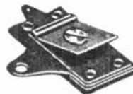
Standard type illustrated at left, popular model for neutralizing, balancing and trimming. Mica dielectric — phosphor bronze flexible plates, bakelite base 1 1/4" x 1 1/16".
