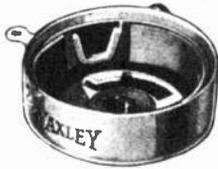
**NEW SPRING WEDGE**—Yaxley Wire Wound Controls embody a new spring wedge design, which definitely eliminates any possibility of loose terminals. Expansion and contraction due to temperature changes are taken up by this patented spring which holds the element and terminals firmly in place.
