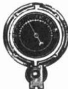
No. 125 Crowe Friction Drive Airplane Dial for Small Receivers—Diameter of scale 2". Ratio 3 1/2 to 1 in 360°. Double-end pointer, 4-channel kilocycle calibration. Black or peach. Convex glass and bronze escutcheon. List Price.....\$1.50
