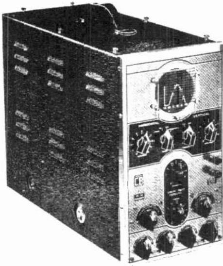
This instrument offers complete facilities for countless problems of receiver circuit study and adjustment. R.F. and I.F. alignment, resistor, condenser, and vibrator tests are made while the receiver is under actual operation.
