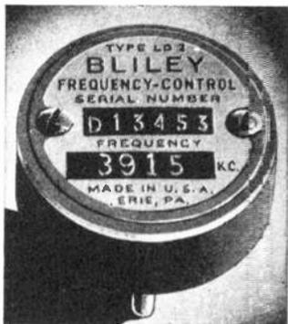
The type LD2 amateur frequency crystal is a mounted, precision low drift crystal for the 80 and 160-meter amateur bands. The crystal is carefully cut from selected Brazilian Quartz, ground to exacting precision, accurately calibrated and rigidly tested. It possesses unusual activity and has a frequency drift of less than 4 cycles/MC./°C.
