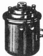
6-8 volt field excitation. 1.0 ampere consumption at 6 volts. 15-ohm voice-coil impedance at 1000 cycles. Continuous operating capacity 25 watts. Peak load capacity 50 watts. Particularly adapted for theatre and auditorium use where the finest quality reproduction is required. Wt. 20 lbs.
