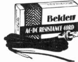
To determine the proper a-c—d-c line cord, add the filament voltages of the individual tubes in the receiver. From the chart below select the nearest figure under the heading SUM OF TUBE VOLTAGES in the column headed by the line voltage of the available power supply.
