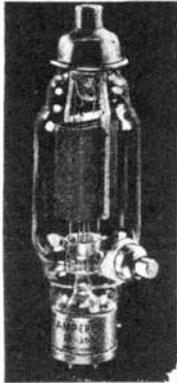
R. F. power amplifier, oscillator, class B modulator.
