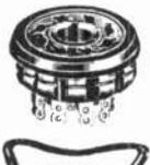
Cadmium-plated contacts, made of brass alloy with two ears for soldering; maintains firm, low resistance contact with tube prongs. Sockets held to chassis by tempered steel ring. No rivet is necessary. Fits any chassis from 0.80 to 0.65 inches thick.
