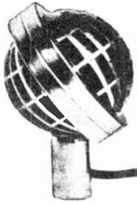
The C-5, a non-directional microphone, recommended for good quality audio pick-up, which includes general public address applications, disc and film recordings, and good amateur phone transmission. The high internal capacity of the dual-crystal elements lowers the impedance proportionately, thus the cable effect is minimized. The frequency response of the C-5 is uniform for all angles of approach. Standard reference level. —68 db. Push-pull or, single grid input may be used.
