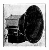
2730 ohms D.C. field. Without output transformer. Diameter of cone, 9". Complete with connecting cable and terminal strip. Very rugged construction and suitable for replacement in other sets and for public address installations.
