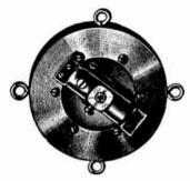
A rugged two button microphone, built of only the finest material obtainable, with a very minimum of hiss. This unit uses a duralumin dia-phragm .002 thickness, with pure gold contacts below each button, the same diaphragm as you obtain in the large A-1
