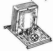
Here is a unit that has been looked for far and wide and is finally presented to you as an efficient field exciter. Uses one 280 tube as rectifier, giving an output of 110 mils at 100 volts. It is suitable to use this to run either dynamic speakers or dynamic units.
