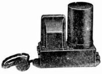
MIK 80 is designed for use solely with PAM 80. Taking advantage of the high amplification of PAM 80, it requires no tubes. It comes equipped with a cord and plug for attachment to PAM 80. through which it gets its power supply. It operates entirely from ac., including button current supply. A 1000-ohm variable volume control is provided, but not built into the unit for the sake of portability and convenience. Terminals for the microphone are tip jacks, color coded.
