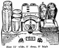
A 6 tube receiver especially designed for the reception of short-wave television broadcasts.
