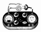
For measuring capacities of paper and electrolytic condensers. A very handy instrument for the radio service shop. Checks paper condensers from .008 to 10 mfd. and all capacities in electrolytic condensers. D.C. voltage for electrolytic testing is obtained from the plate of a rectifier tube by use of a special adapter. Housed in a neat metal case with or without cover.
