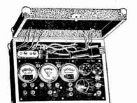
A complete, accurate and reliable analyzer and circuit tester. One of the most popular set testers ever built. Equipped with an improved type selector switch for testing all parts of the tube circuits by plugging into the sockets of the set under test. Selection for testing filament, plate, grid and cathode voltages is accomplished quickly and accurately.
