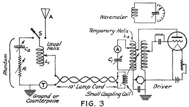
CONNECTIONS FOR ANTENNA RESISTANCE MEASUREMENTS
