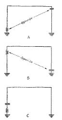
FIG. 1 CONVERTING AN ANTENNA INTO A LOOP
