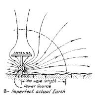
FIG. 1 - FLOW OF POWER FROM AN ANTENNA
