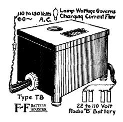
be disconnected from the set before charging, as the D.C. circuits are not insulated from the A.C. end of the rectifier. An extension cord and plug makes connection to 110 V. A.C. line, and two clips with their polarities marked are used to connect to the battery terminals.
