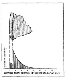
FIG. 5 Showing current distribution in a No 18 B.&S. copper wire with a nickel-plated surface - (200 meters)
