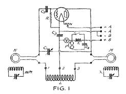
375 meters. Other ranges may be secured by substituting other coils. The two exploring coils M and N are made of four turns of No. 18 annunicator wire with 16-inch leads which are solidly tapped together. C<sub>1</sub> is a variable condenser of .001 microfarad maximum capacity; C<sub>2</sub> is a
