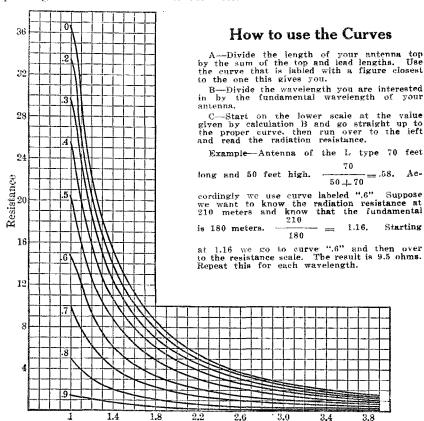
Figure 2 Radiation Resistance Curves for Reading Radiation Resistance Offhand
