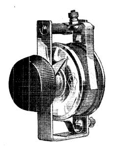
This potentiometer is of the revolving drum type and the resistance unit has a resistance of 300 ohms. The resistance wire is clamped between two insulated caps which hold the wire firmly in a horizontal position. The broad, flat contact on the tightly clamped resistance unit insures that the wire will not be damaged or displaced under constant usage. The instrument is designed for panel mounting and is provided with three binding posts to facilitate wiring.
