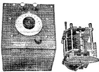
Fig. 5-Laboratory Type Variable Condenser
