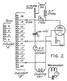
cycles (100 to 475 meters) and inductor B is used when frequencies from 1,000 to 100 kilocycles (300 to 3000 meters) are desired. The small coil A consists of 24 turns of No. 18 B. & S. gage D.C.C. wire wound on a tube 3½ inches in diameter and about 2½ inches long. The space occupied by the winding is about 1% inches.
