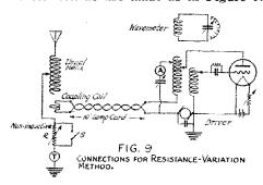
The thermo-galvanometer is the same sort of an instrument as before, the resistance R may be a decade resistance or simply a ten-foot length of No. 30 B.&S. gage resistance wire with a sliding contact, such as a clip. If a powerful driver (over 20 watts) is used a less sensitive instrument may be used at T. Keep the driver at least ten feet from the helix and insert the small coupling coil in series with the ground side of the oscillating circuit.
