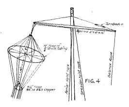
The down-lead cage was made small in size to concentrate the capacity at the top. Hoops of No. 10 hard drawn copper were used, spaced, 6 feet apart. The top was assembled first, then a 10 foot hoop and a 6½" hoop were soldered in position as shown in Figures 4 and 5, this being done with the whole hanging vertically.
