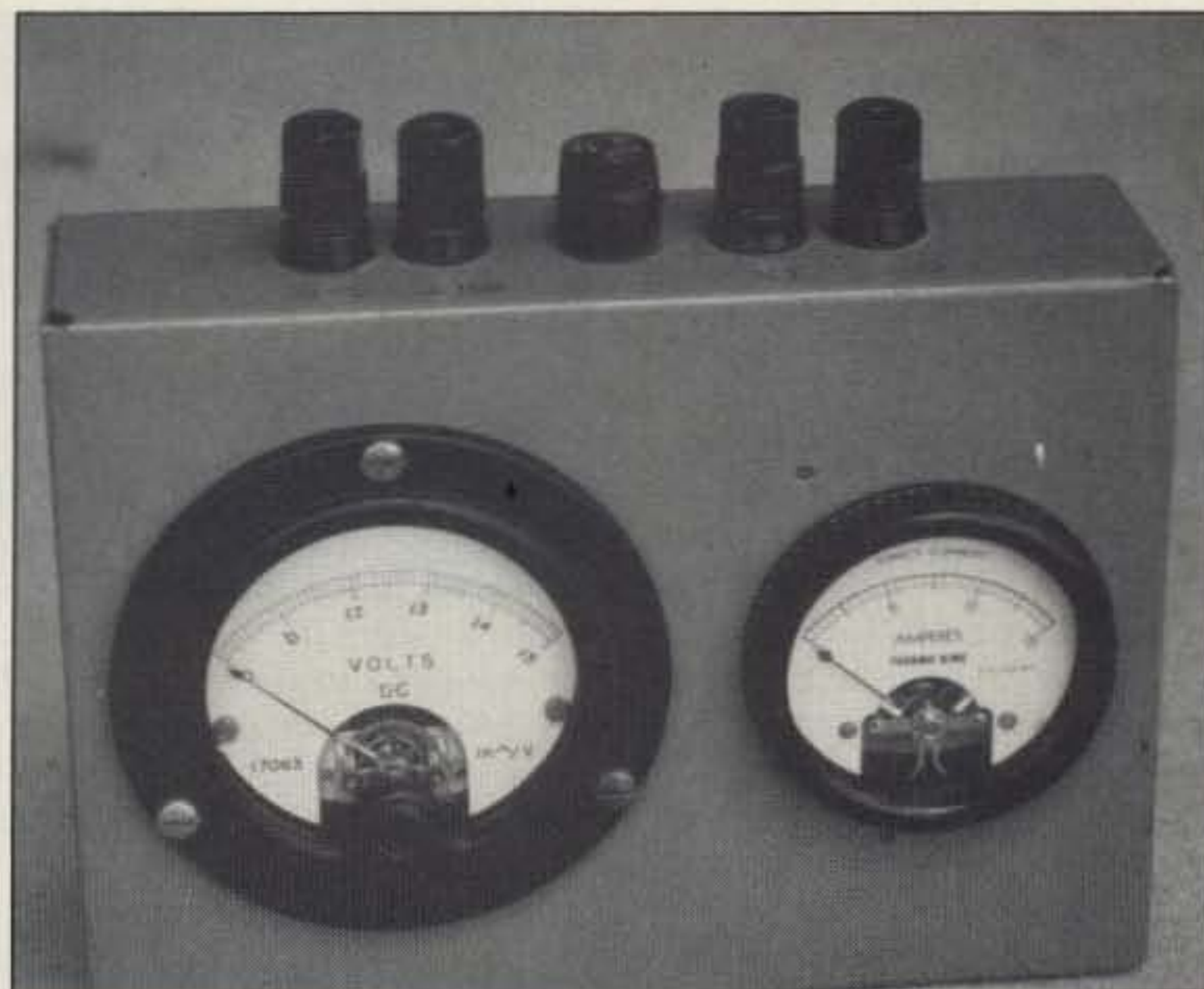
Photo C. Another example of an expanded-scale voltmeter. This unit includes a series ammeter to monitor charging current.
