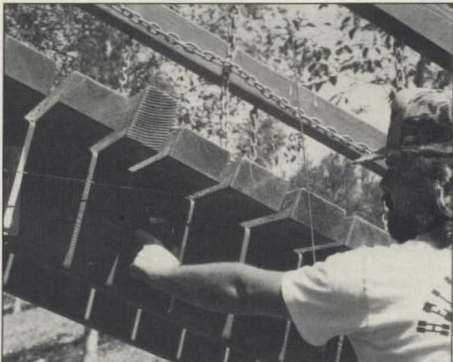
Photo C. Many hunters, including Jerry Hughes KC6YMP, were certain that this tagged horizontal mag-mount antenna belonged to the hidden T. But its coax was not hooked up. The actual emitter was the chain, just inches away.
