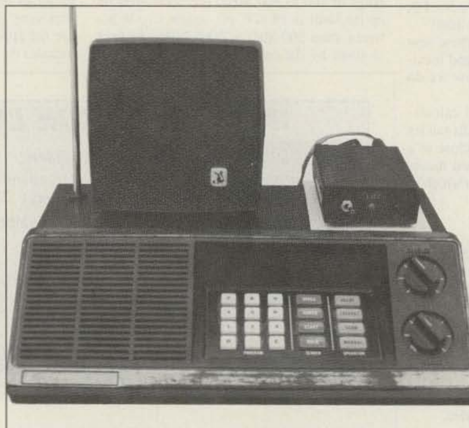
Photo B. The LiTZ (Long Tone Zero) decoder in service using a flea market scanner and mobile speaker.
