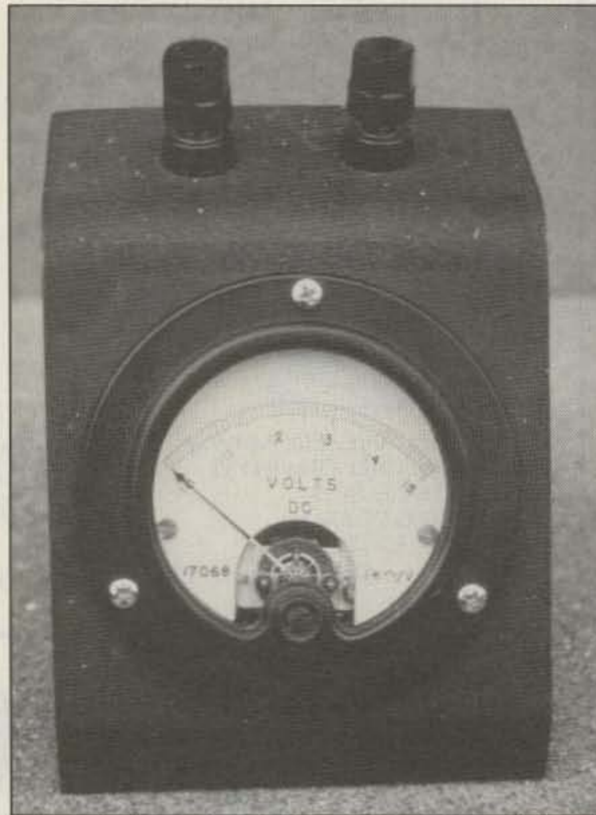
Photo A. Front view of a completed expanded-scale voltmeter, mounted in a metal case. The original 0-5 volt DC meter was modified by inking a "1" before each digit.
