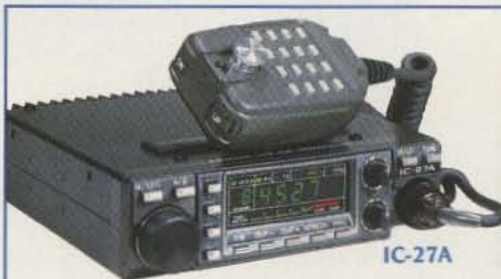
The IC-27H 45 watt and IC-27A 25 watt ultra compact 2-meter mobiles continue to be available.
