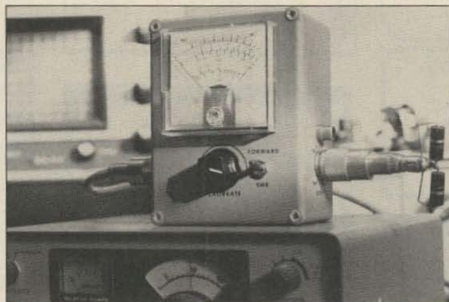
Photo A. The QRP swr/wattmeter shown with the HW-8, built using junk-box parts.
