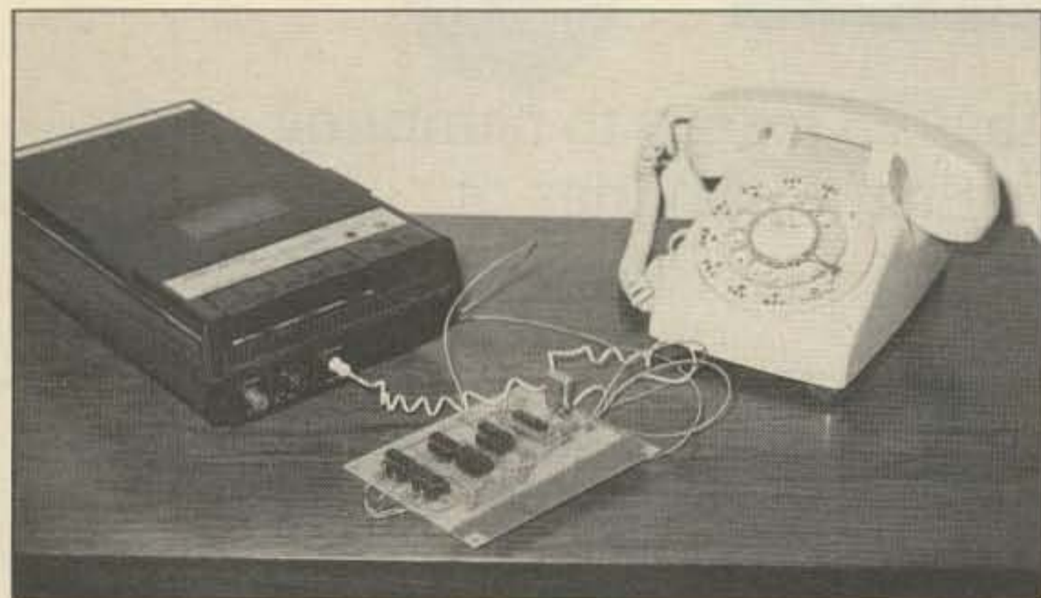
Photo A. The remote-control system, wired and waiting for a call.
