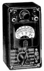
SPECIFICATIONS: 6 A.C. VOLTAGE RANGES: 0-15/30/150/300/1,500/-3,000 Volts. 6 D.C. VOLTAGE RANGES: 0-71/2/15/75/150/750/1,500 Volts. 4 D.C. CURRENT RANGES: 0-11/2/15/150 Ma.; 0-11/2 Amps. 2 RE-SISTANCE RANGES: 0-500 Ohms; 0-1 Megohm.
