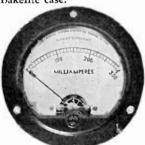
3" ROUND CASE—OPEN FACE STYLE. Flange diameter, 3½"; depth overall, 2½"; body diameter, 2¾"; scale length, 2-9/16". Bakelite case.
