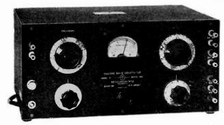
R. F. MODULATOR: 5 volts maximum carrier input. Translation gain is approximately unity—Output impedance is 600 ohms.
