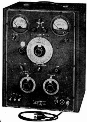
Distortion: FM distortion at 75 kc. deviation is less than 2% when modulated with the internal AF oscillator or an external AF oscillator having 0.5% distortion or less. At 50% amplitude modulation the distortion is about 5% using the internal AF oscillator and decreases as the modulation percentage is reduced. An external AF oscillator may be employed for amplitude modulation if desired.
