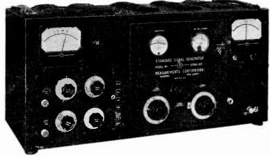
POWER SUPPLY: 117 volts, 60 cycles. 230 watts (with regulator). DIMENSIONS: 12" high x 26" wide x 10" deep, overall. WEIGHT: Approximately 135 pounds, including external line voltage regulator.
