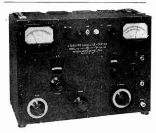
LEAKAGE AND STRAY FIELD: Less than 1 microvolt from 80 kilocycles to 50 megacycles.
