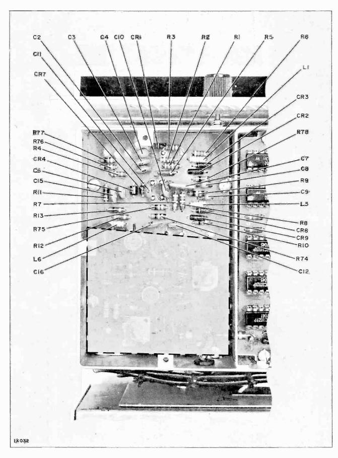
Figure 19. Exciter, Modulated Oscillator Board, Parts Location
