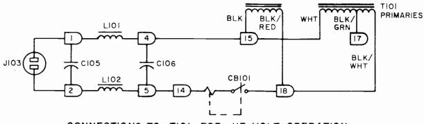
CONNECTIONS TO TIOI FOR 117 VOLT OPERATION
