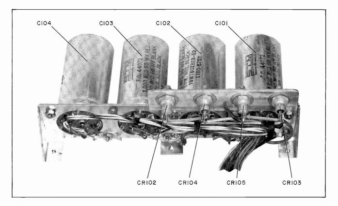
Figure 12. Main Frame, Rectifier and Filter
