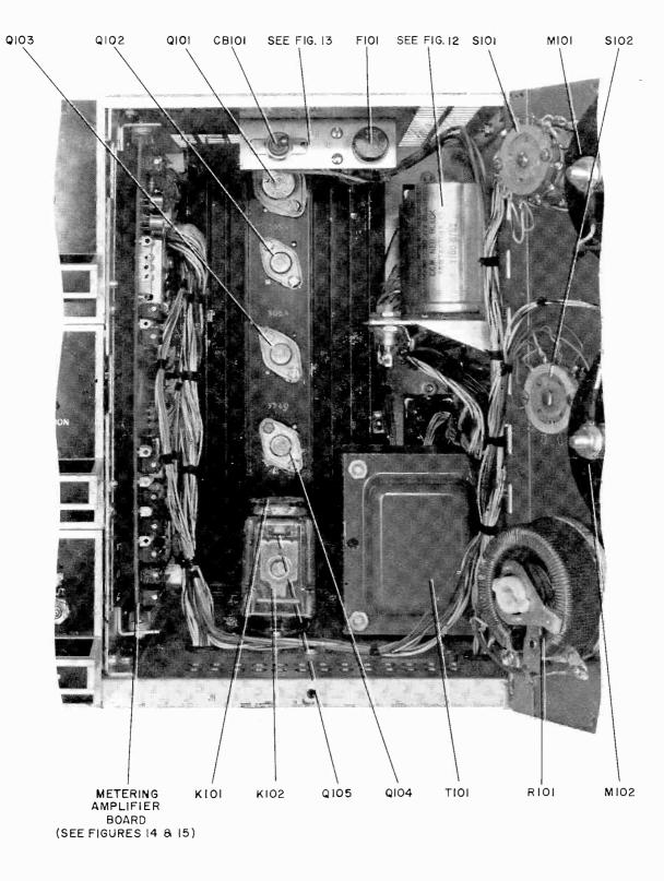
Figure 11. Main Frame, Parts Location
