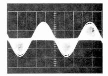
TP314 (gray); 55 kHz Filter Output .1 V/cm, .5 ms/cm Sync: Ext. audio generator
