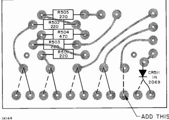
ADD THIS JUMPER TO ENABLE TELEMETERING TONES TO BE APPLIED TO SUBCARRIER
