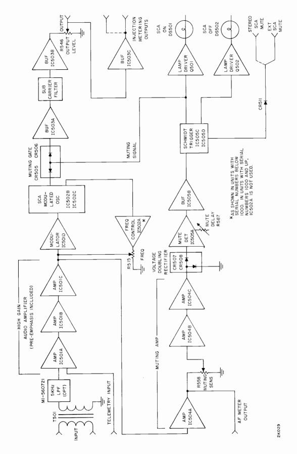
Figure 5. BTX-1B SCA Generator, Simplified Block Diagram
