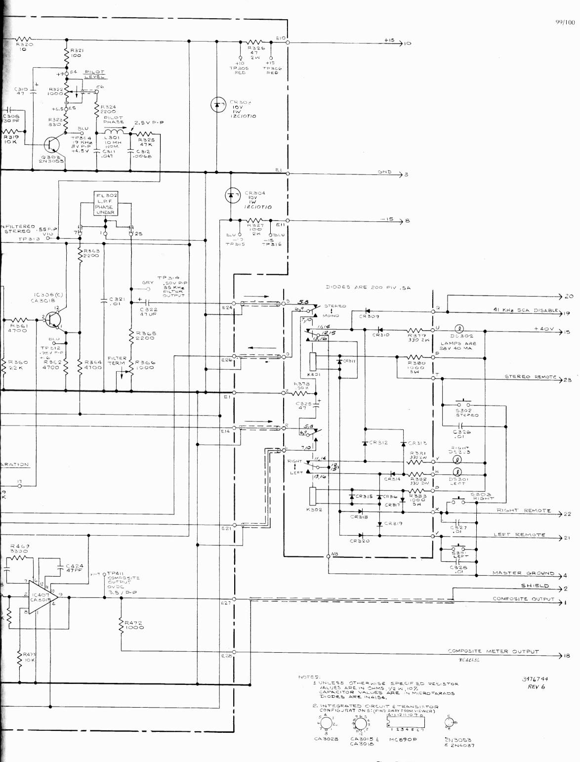
Figure 52. BTS-1B Stereo Generator, Schematic Diagram
