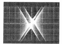
TP411 (white); Composite Output .1 V/cm, 50 μsec/cm Sync: Ext. audio generator Photo to left expanded to show waveform when pilot phase is misadjusted.
