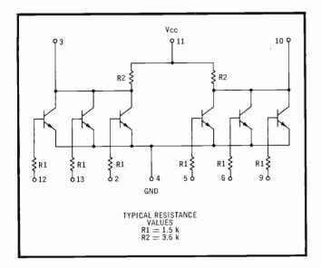
Two 3-input positive logic NOR gates in a single package. Each may be used independently, paralleled for increasing the number of inputs (subject to loading rules), or cross-connected to form bistable elements.
