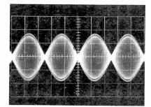
TP411 (white); Composite Output 1 V/cm, .5 ms/cm Sync: Ext. audio generator Normal L-R waveform
