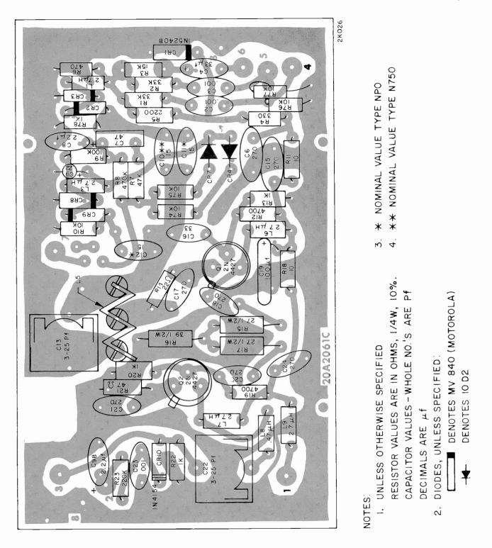
Figure 25. Exciter, Modulated Oscillator Board, Parts Overlay, Bottom
