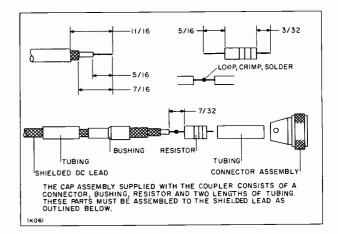
Figure 68. Connector Cap Assembly Details
