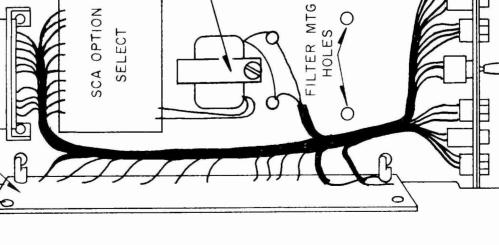
Figure 57. BTX-1B Low Pass Filter Installation
