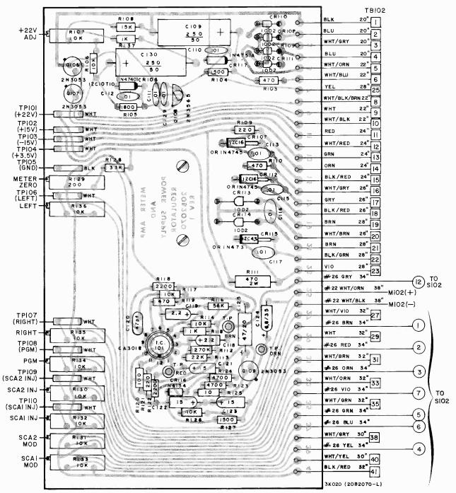
NOTE: UNLESS OTHERWISE SPECIFIED, RESISTOR VALUES ARE IN OHMS, 1/2 WATT, 10%. CAPACITOR VALUES ARE IN MICROFARADS.
