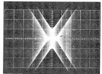
TP411 (white); Composite Output .1 V/cm, 50 μsec/cm Sync: Ext. audio generator Photo to left expanded to show waveform when pilot phase is properly adjusted.
