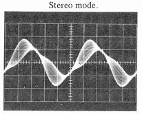
TP411 (white); Composite Output .1 V/em, 10 µsec/cm Sync: Ext. from TP304 Left only input at J109; audio level set for 15% modulation of carrier, including 9% pilot. This waveform may be used to identify the left channel.
