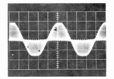
TP411 (white); Composite Output 1 V/cm, .5 ms/cm Sync: Ext. audio generator Waveform showing effect of extreme overmodulation; input level increased to give more than 200% modulation.
