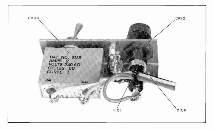
Figure 13. Main Frame, Fuse Panel
