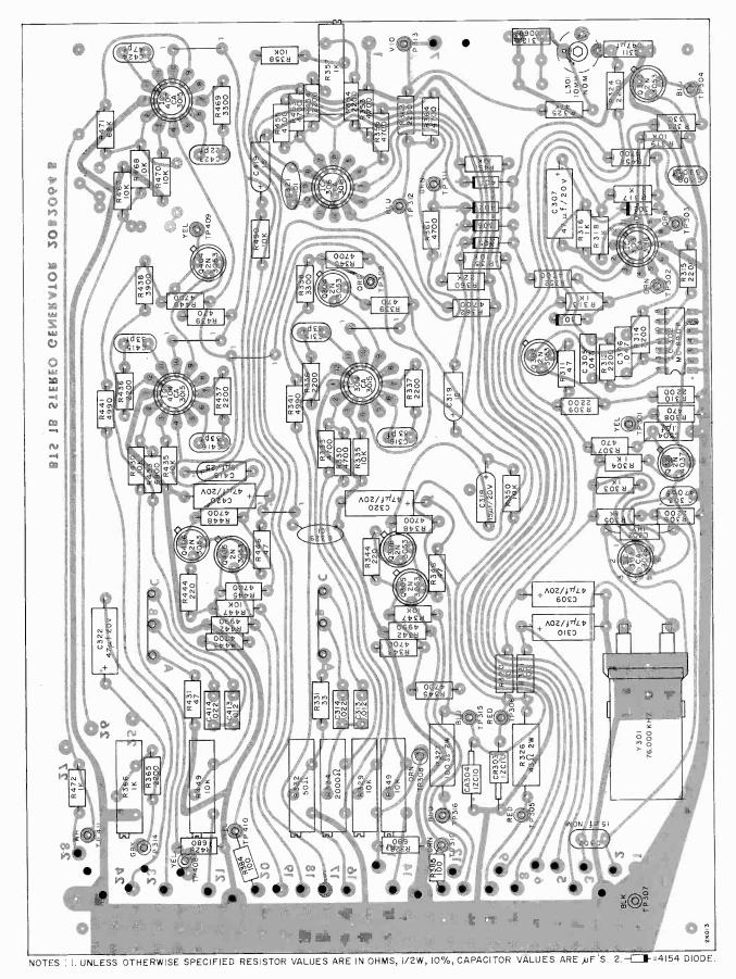
Figure 34. Stereo Generator Board, Parts Overlay, Top
