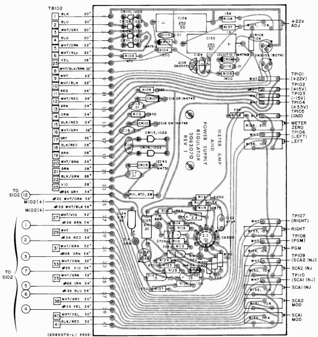
NOTE: UNLESS OTHERWISE SPECIFIED, RESISTOR VALUES ARE IN OHMS, 1/2 WATT, 10%. CAPACITOR VALUES ARE IN MICROFARADS.
