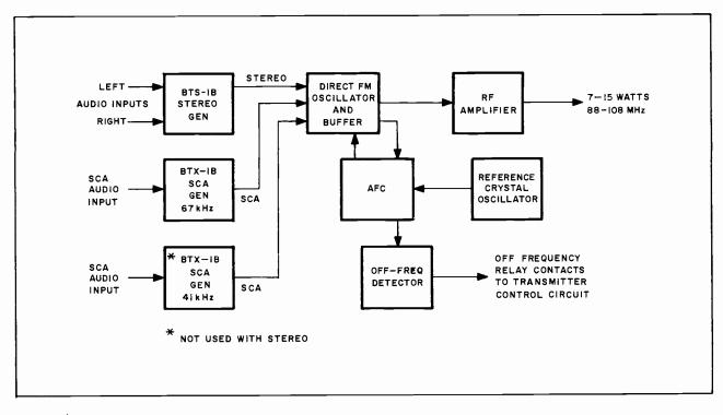
Figure 2. BTE–15A System, Block Diagram
