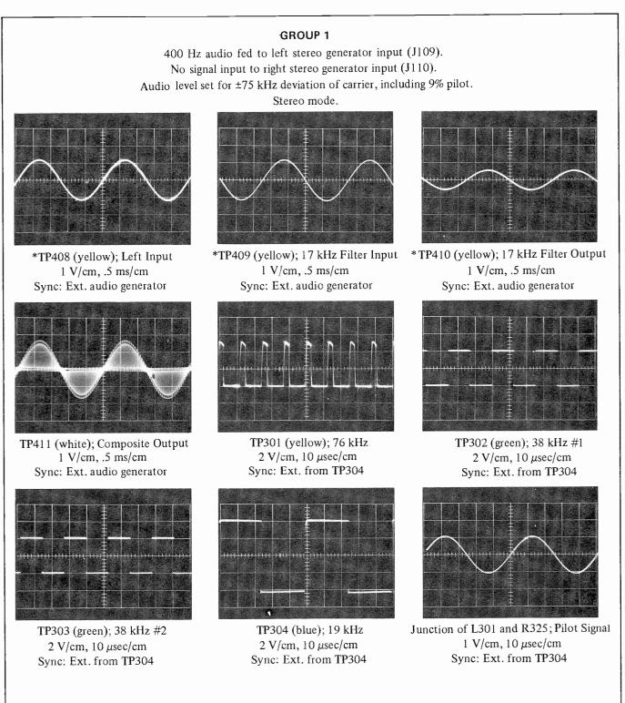
\*With a signal input to the right stereo generator input (J110), these waveforms will appear at TP308, TP309 and TP310.
