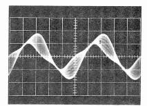
TP411 (white); Composite Output .1 V/cm, 10  $\mu$ sec/cm Sync: Ext. from TP304 Right only input at J110; audio level set for 15% modulation of carrier, including 9% pilot. This waveform may be used to identify the right channel.
