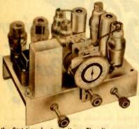
S HORT-WAVE "DX" fans will especially appreciate the new Trutest 6-Tube "Skip Band" receiver kit, for it takes in nat only the entire domestic broadcast band from 200 to 550 meters, but the important fareign channel from 17.6 to 50 meters as well. It is so easy to assemble and wire that even a novice can do the job and have the set work
