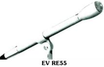
The flat response from 40 to 20,000 Hz, and omni-directional polar pattern of the RE-55 make it a favorite for single pair stereo recording. Free of distortion at sound pressure levels approaching 160dB.
