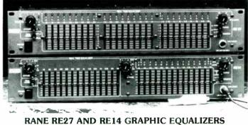
These combination graphic equalizers and realtime analyzers make tuning a room simple, quick and accurate. The three LED display with either  $\pm 3$ dB or  $\pm 1$ dB range is used with the supplied flat response mic and built in pink noise source. Unplug the mic, and the display monitors program through the equalizer section to aid in pinpointing feedback. The EQ sections are similar to the GE27 and GE14 above: the separate RA27 Analyzer is described on page 55. **RE27 ONE THIRD OCTAVE EQ**
