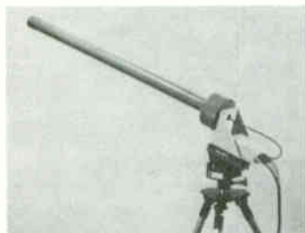
Point to Point Microwave Antennas
