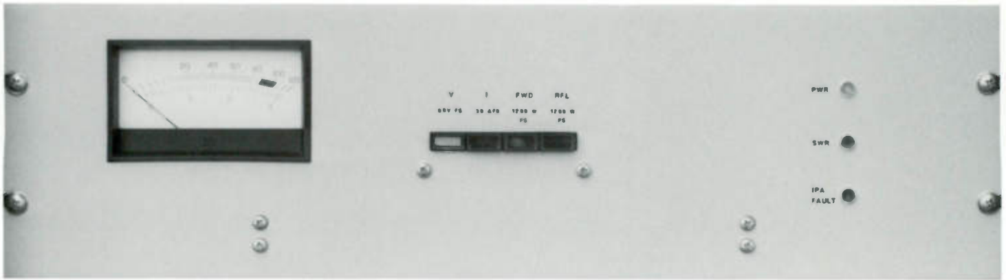
Above: close-up of solid-state driver control panel from in front of the transmitter.
