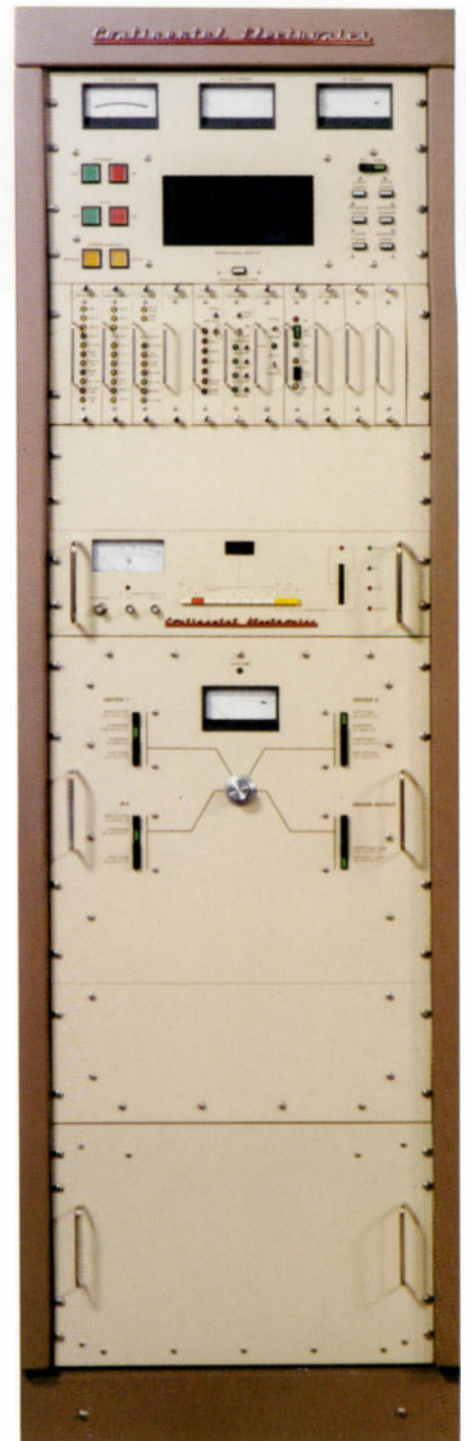
Above photo: the Control and Driver Unit houses the Type 802A FM Exciter, IPA and Driver Units, transmitter control and monitoring.
