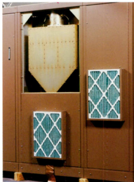
Rear view of transmitter Cavity Unit with cover removed shows self-contained harmonic filter.
