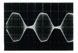
FIGURE 2-8 UNDER-CORRECTED MODULATION ENVELOPE (Tilt Present)
