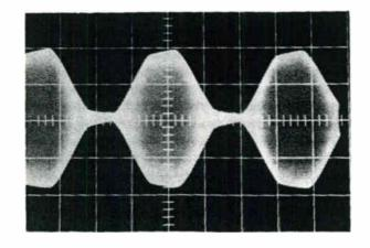
FIGURE 2-9 OVER-CORRECTED MODULATION ENVELOPE
