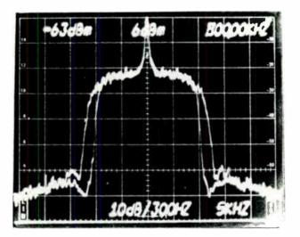
FIGURE 3-1 TYPICAL TRANSMITTED SPECTRUM COMPARISON (9.5/11 kHz Bandwidth Selection, 15 minute peak-store display; V:10 dB/div, H: 5 kHz/div., 300 Hz resolution; monaural program).
