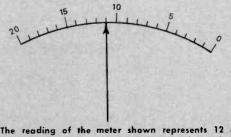
Fig. 2—The reading of the meter shown represents 12 ohms on the R X 1 scale, 120 ohms on the R X 10 scale, and so on up to the R X 1000 scale.
