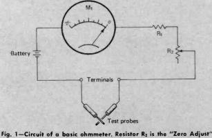
Fig. 1—Circuit of a basic ohmmeter. Resistor  $R_2$  is the "Zero Adjust" control. The resistance to be measured must be connected between the tips of the test probes.
