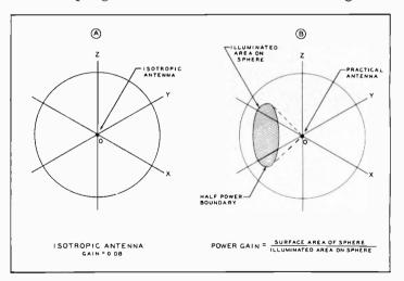
Figure 2—The isotropic antenna, which is the point of reference for antenna measurements, is an antenna which radiates equally well in all directions. A representation of an isotropic antenna could be a pinpoint of light (0) placed at the exact center of a hollow globe (illustration A). The light will illuminate the inside of the globe uniformly.
