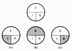
Fig. 2.14—The Ohm's Law circle can be used until the formulas are memorized. Covering the unknown symbol leaves the proper formula exposed.
