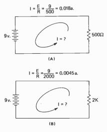
Fig. 2.11(A)—With 9V applied to a 500 ohm resistance Ohm's law indicates a current flow of 0.018A. (B) With the voltage held at 9V but R increased to 2K the current drops to 0.0045A. This shows an inverse relationship between I and R.
