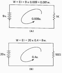
Fig. 2.15—Typical wattage dissipation calculations. In (A) the resistor actually dissipates 0.081 watts. A safety factor of 100% requires a rating of 0.162 watts. The closest practical rating would be 1/4 watt. For problem (B) where the calculations show 8 watts, the 100% safety factor brings the required rating to 16W. Only a 15 or 20 watt rating would be available and 15W would be adequate.
