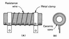
Fig. 2.6—Construction of a typical wirewound resistor.
