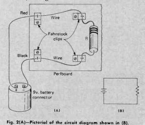
Remember, to convert mA to A move the decimal point three places to the left. Compare the calculated value of R with the measured value.
