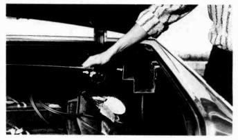
passed durability. It is constructed of 12-gauge, coldrolled steel, and is coated with zinc chromate. The hinge is of stainless steel, and is spot-welded to the clamp to provide positive ground contact. In addition, the hinge is fitted with a stop which holds the antenna suspended and off the trunk floor while stored, allowing for short-range reception from inside the trunk.
