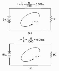
Fig. 2.10(A)—When 9V is applied to a 1 K resistance the current flow according to Ohm's law will be 0.009A. (B) When the voltage applied to the resistance is increased, the current flow will increase.
