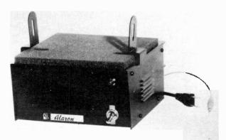
For using Mobile CB Transceiver as Base unit. Converts 117 v AC current to 13.8 DC. Solid State. Built-in powerful 8 ohm speaker, one 3 amp DC and one 2 amp AC fuse, On/Off switch, pilot light, speaker connector cable with plug, UL approved AC cord, DC output power terminals with screw on caps. 2 adjustable spring brackets hold Mobile CB to top of Power Supply and let it slip out by simply lifting CB off. All metal cabinet. Individually boxed.
