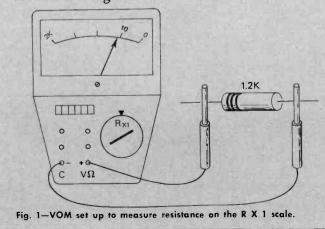
4-Read the resistance value from the ohmmeter scale. Note that the reading is at the extreme left end of the scale and cannot be read accurately.
