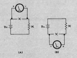
Fig. 3—To place a milliammeter in series with a circuit it is first necessary to break the circuit. Since the current flow is the same at any point in a series circuit, the meter may be inserted at any point, as shown in (A) and (B), and it will produce the same reading. capable of reading as high as 600 mA in four ranges.
