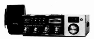
Employing both a fully variable Noise Limiter and a Switchable Noise Blanker, the Sabre will let the operator adjust its quieting to any man-made or atmospheric conditions for maximum signal reception.
