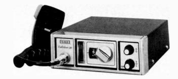
lation and signal strength of received stations. It operates on 13.8VDC, with either a positive or negative ground, but it can also be operated on 117 VAC with an optional accessory power pack (SBE-1AC) available from SBE.
