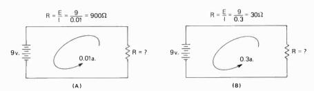
Fig. 2.13(A)—When the voltage and current are known Ohm's law may be used to determine the circuit resistance. (B) The resistance in a circuit must decrease in order for I to increase (assuming a constant voltage).
