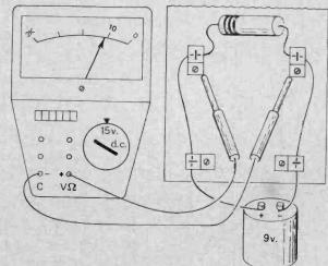
Fig. 3-Measuring the voltage drop across the 1K resistor.
