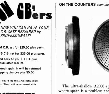
The ultra-shallow A2000 speakers can be used anywhere space is a problem and quality sound reproduction, along with power handling capability, is a requirement. These low-distortion high-fidelity speakers handle a full 10 watts RMS of power over a frequency range of 70 to 20,000 Hz. Input impedance is 4-8 ohms.
