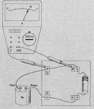
Fig. 4—Measuring the current flow through the 1K resistor.
