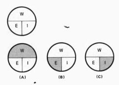
Fig. 2.16—The wattage circle that can be used until the formulas are memorized. Covering the unknown symbol leaves the proper formula exposed.
