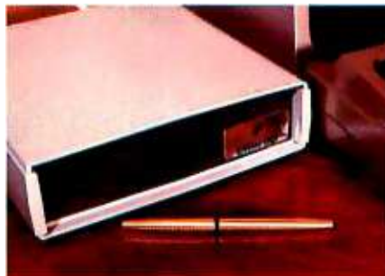
Photo 1: The Disk-80 mounted in its enclosure and attached to the TRS-80 Model I computer. The Disk-80 is about half the size of the Radio Shack TRS-80 Expansion Interface.
