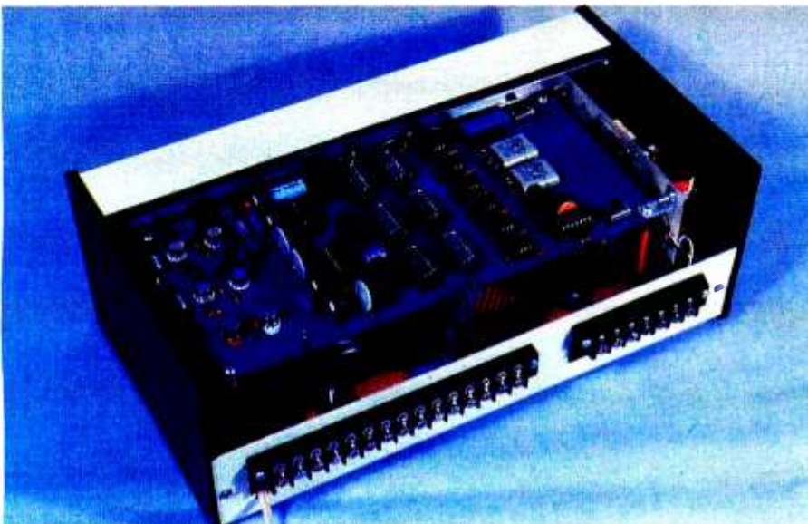
Photo 5: An internal view of the I/O controller containing relays, optoisolators, and analog interface components.
