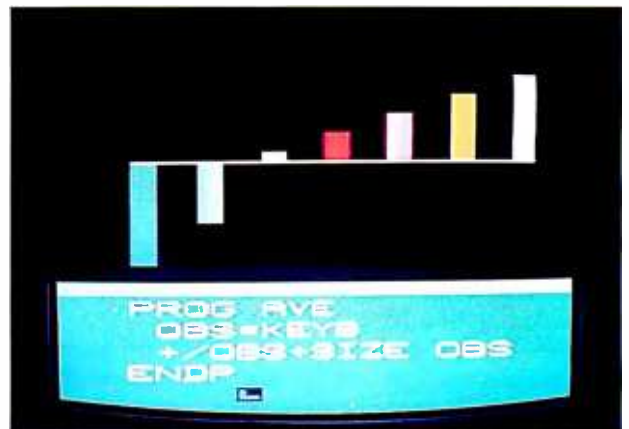
Photo 2: Program AVE, which computes the average of a set of numeric observations. Input is from the keyboard as a series of numeric values — an array constant. The input, returned by the KEYB function, is assigned to OBS, thus making OBS an array. The average value is computed by adding up the elements of the array (+/OBS) and dividing the sum by the size of the array (SIZE OBS). Since the result is not assigned to a variable, it is displayed.
