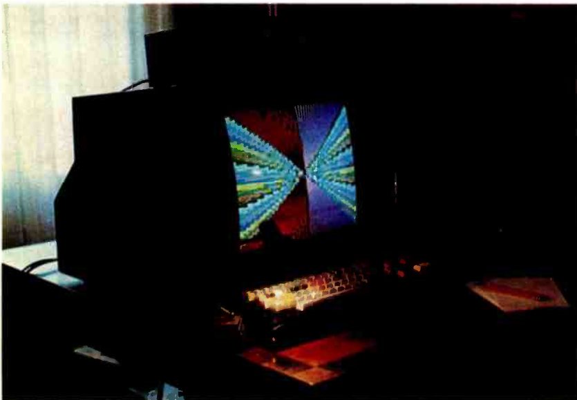
Photo 1: The Compucolor 8051 with extended ASCII keyboard and "floppy tape" storage. The tapes are similar to 8 track music cartridge tapes, except that they are shorter. More recent models use a floppy disk system for storage.
