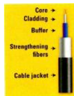
Figure 1. A fiber cable is made up of five elements beginning with the core, where light passes through, out to a jacket normally made of PVC.
