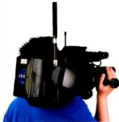
Shown here is a BMS HD transmitter hidden inside the pictured Sony camera's right-side cam shell. Photo courtesy BMS.
