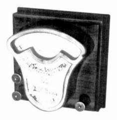
KNOTT STUDENT'S AMMETER - This beautiful example of laboratory equipment was manufactured by the L.F. Knott Apparatus Co. of Boston. The thick mahogany board, heavy metal casting, and rugged binding posts helped it survive rough handling in the laboratory since the early 1900s. (Dave Crocker - Mashpee. MA)
