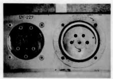
Figure 5. Note that the socket on the right is mounted using four screws rather than rivets, as is the socket on the left and all other tube sockets in the set
