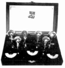
A-C-S RADIO RECEIVER – This compact 6-tube radio was manufactured by the Multiple Selling Corp., Madison Ave., New York City. It features "No Solder" electrical connections using copper strips. Its size, wth cover closed, is 7" x 13" x 7"/4". It has many similarities, especially the dials, to that of the Martian "Beauty" 1-tube set. If anyone has any information about this receiver or the manufacturer, please write A.R.C. (Ed Bell – Raleigh, NC)
