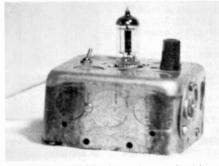
The line-operated 1-tube radio contained in an electrical junction box.
