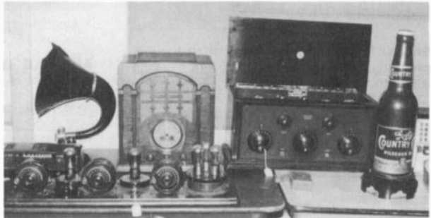
Awaiting auction: an Atwater Kent Model 10 breadboard, a Burns horn speaker with broken petals, a Gilfillan Neutrodyne and a Goetz beer bottle radio.
