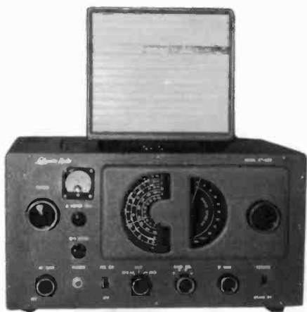
LAFAYETTE MODEL KT-200 – The dials on this Japanese-made communications receiver appear to be identical to the dials on a Hallicrafters Model S-38B. The number of bands (4) and the tuning range (.54 to 32 MHz) are also the same. However, the S-38B is an AC/DC set, while the KT-200 is AC, using tube Types 6BD6 (3), 6BE6 (2), 6AV6 (2), 6AR5 (1), and 5Y3 (1). The Lafayette is pictured with an optional external speaker, HE-11, which is a later piece of equipment sold in the early 1960s. (Doug Burskey – Mansfield, OH)
