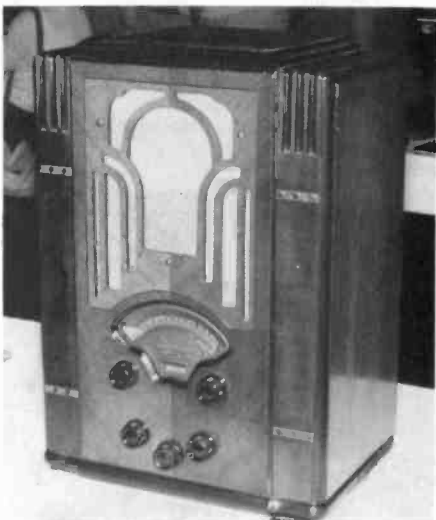
This is a 9-tube Atwater Kent Model 649, which is possibly the last of the "fan" dials.
