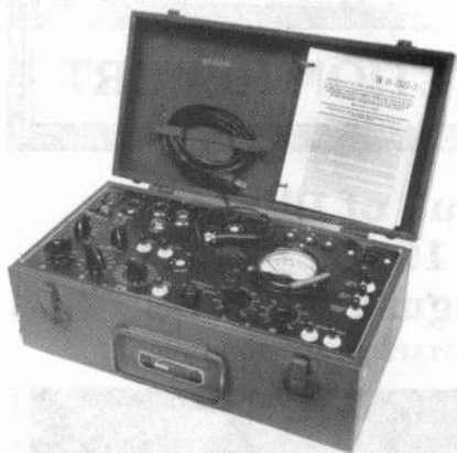
Figure 3. The I-177A tube tester, complete with instruction manual. The date stamped on the inside cover of the case reads "MFP August, 1949."
