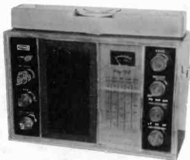
RAYTHEON MODEL RAY-DF – This unusual transistor radio was made in Japan and has 5 bands (AM-FM-VHF-MF-LF) with "DF" level meter and BFO. It also has a directional finder on top that turns 360 degrees. The set may have been designed for marine use. (Dave Mock – Montpelier, OH)
