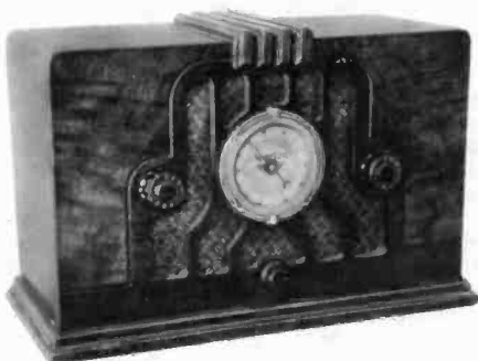
SPARTON MODEL 594 – This attractive little 5-tube AC/DC set uses a resistance line cord to provide the proper voltages for the tube filaments. The finish and the grille cloth are original. (Bill Harris – Roanoke, TX)
