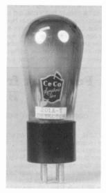
Figure 3. A converted solid-state CeCo Type 201-A tube which can be used as a detector.
