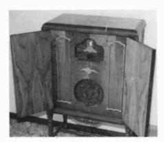
A 1930 Atwater Kent console with a Model 70 chassis, available as AC, DC or battery.
