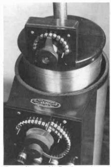
Figure 5. Close-up of the Type 94 receiving transformer tap switches and name plate.
