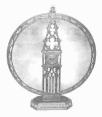
PATHÉ CONE SPEAKER - This lighted Pathé cone speaker is 21" tall and 18" in diameter. There are two lights between the column and cone, and when lit, the column resembles a church. (Don Howland - Spokane, WA)
