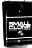
The Small Clone is a full-chorus guitar pedal with a simple, one-knob Rate control and a single
