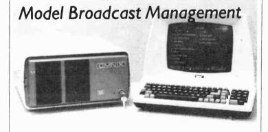
**NIDUS Broadcast Systems** has added two new models to its family of broadcast management automation systems. System 100 utilizes dual floppy disk storage while sister System 110 employs a 5¼ " Winchester hard disk storage. Basic system cost covers hardware, billing, traffic and accounts receivable software, as well as installation/training. Among the software options: accounts payable, payroll, music library, music scheduling, and word processing. Contact (800) 525-0331.
