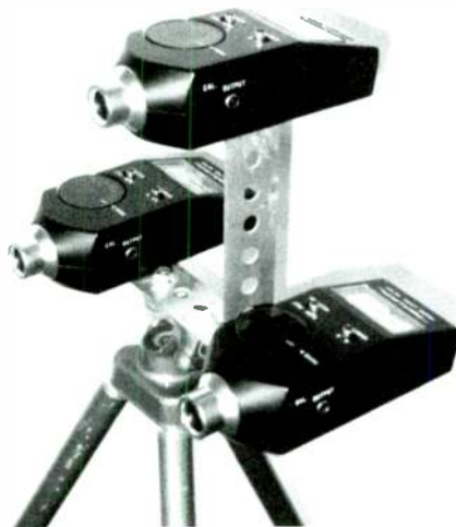
PHOTO 3: The sound-level meters used to measure frequency response. The average of three meters provides a more representative answer. Acoustical measurements at a single point can be very misleading, particularly when they are taken indoors.
