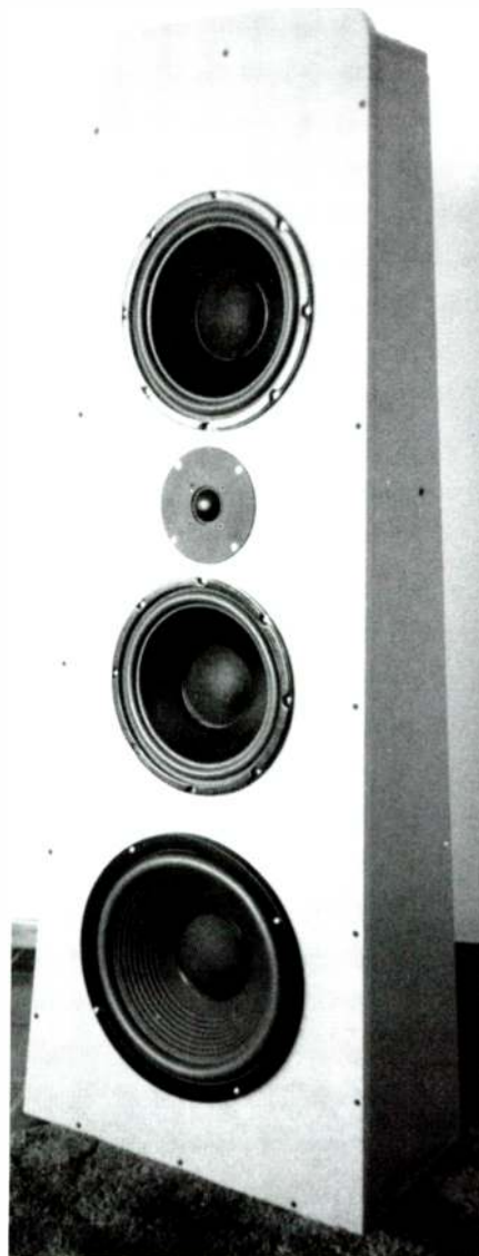
PHOTO 1: The front of the open baffle final prototype, showing the placement of the individual drivers and the side panels.
