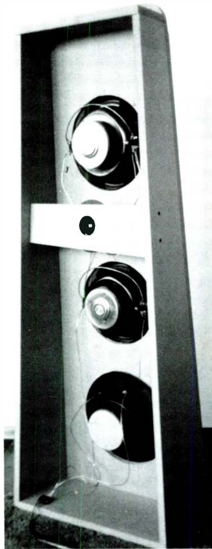
PHOTO 2: The rear of the open baffle final prototype, with the wiring only partially connected.
