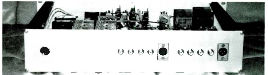
PHOTO 2: Rear view of the crossover. XLR is used for symmetrical, and Teflon ® isolated cinch for asymmetrical input. Note that on this prototype we didn't mount the XLR plug that would be needed for symmetrical output.
