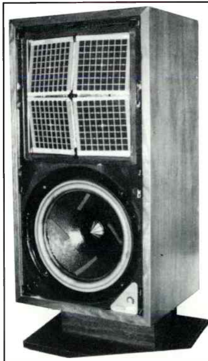
PHOTO 1: Modified Janszen Z412hp now has deep bass response matching the detail and low coloration of the electrostatic elements.
