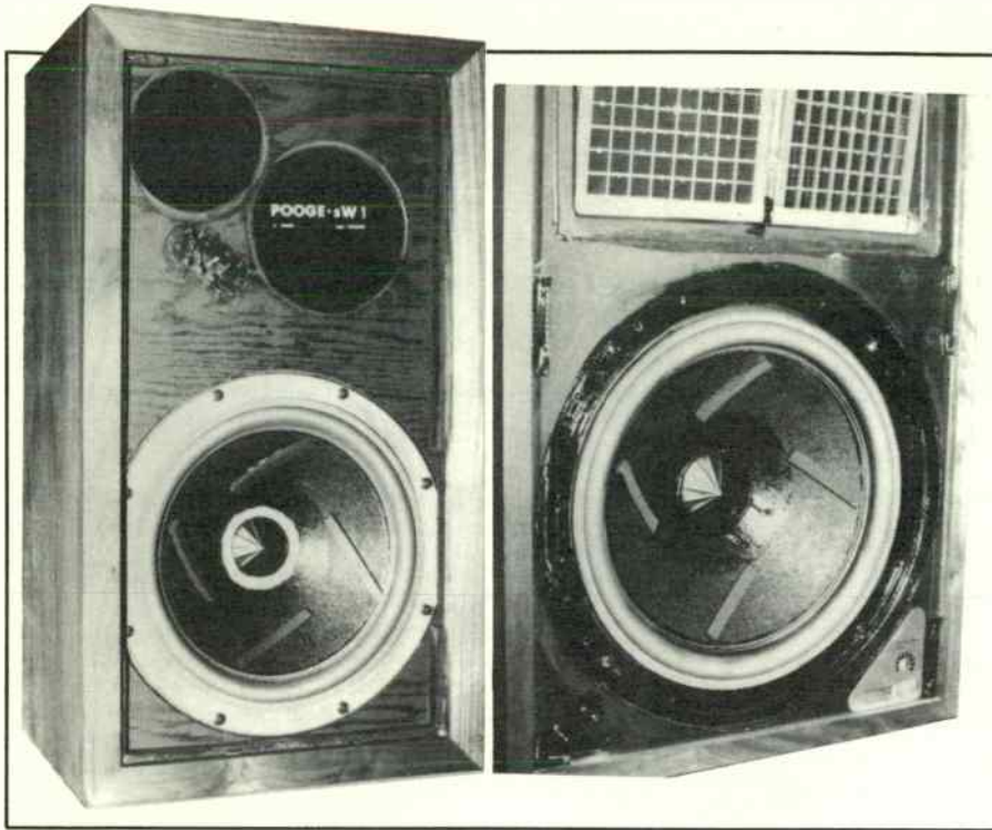
PHOTO 2: Two of these POOGE-SWI subwoofers upgrade the single muddy 18" subwoofer of the Infinity Servo-Static I to reproduce deep bass with the clarity and purity of timbre needed to complement the electrostatic panels.
