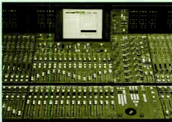
Center console section showing Remote Grouping faders and MixMaster section. Mic input, EQ and aux send sections are at upper right.
