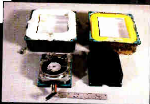
The voice recorder is housed in protective layers inside the recorder box, shown unassembled here.
