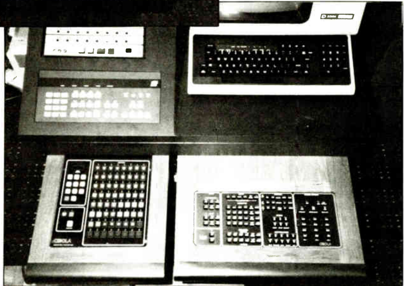
Left pullout drawer: computer controlled routing and assignment switcher. Right drawer: Cibola's multi-function remote controller
