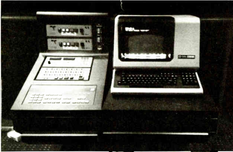
Audio remote control panel; MCI transport remotes, BTX Shadow Synchronizer, data entry terminal
