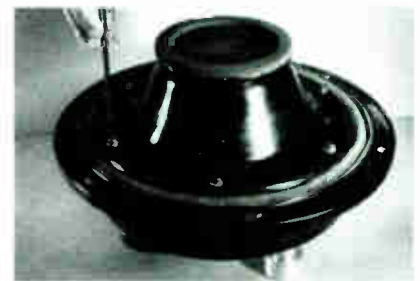
(Right) Featuring a 4 inch diameter throat and a power output of 100 acoustic watts, the M4 compression loudspeaker measures 13 inches in diameter and weighs 38 pounds.
