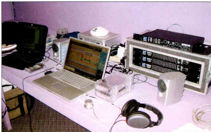
Philip Harvey's tour recording station with PowerBook, Metric Halo units and headphones, among other gear
