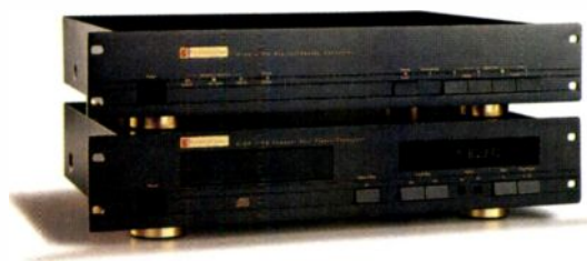
D/AC-1500 and C/DP-1000 The D/AC-1500 is our premier digital to analog converter. The C/DP-1000 is our high resolution CD player. With the simple addition of our Advanced Digital Adaptor Module (an ST optical link), it's transformed into a high performance CD transport.
