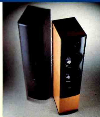
Snell's 42½-inch-high E.5 speaker ($600) has a second tweeter in back.
